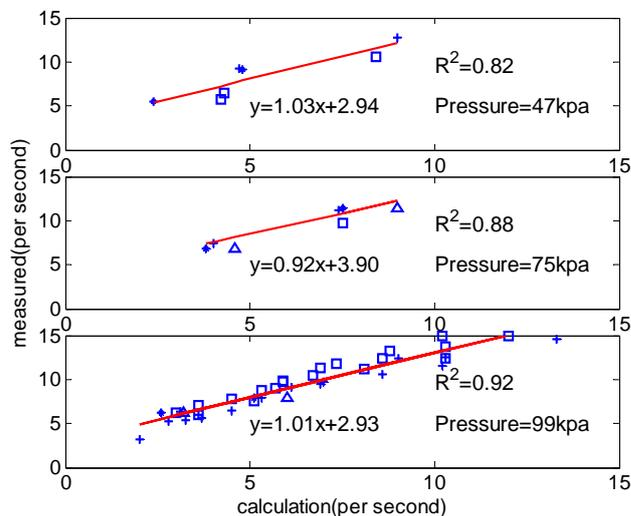
**Fig. 3.** Laboratory calibration for the OH reactivity instrument using different gases at different pressures. The measured OH reactivity is plotted versus the calculated OH reactivity. Calibration gases include CO (hollow square), isoprene (plus sign), propane (star) and propene (triangle).
