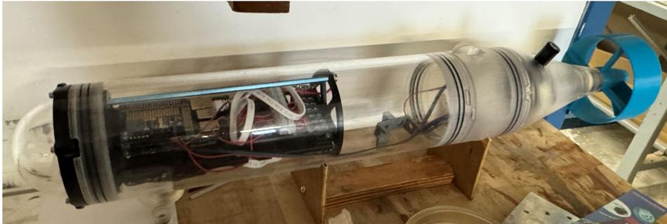
**Figure 3-1:** Short Hulled AUV
