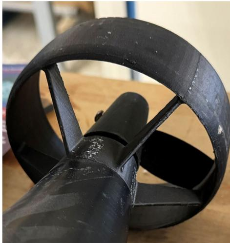
**Figure 2-3:** Example of a single bladed propeller
