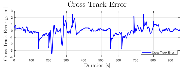
Figure 34: Cross track error for mission presented in Fig. 33, RMS = 0.706909m
