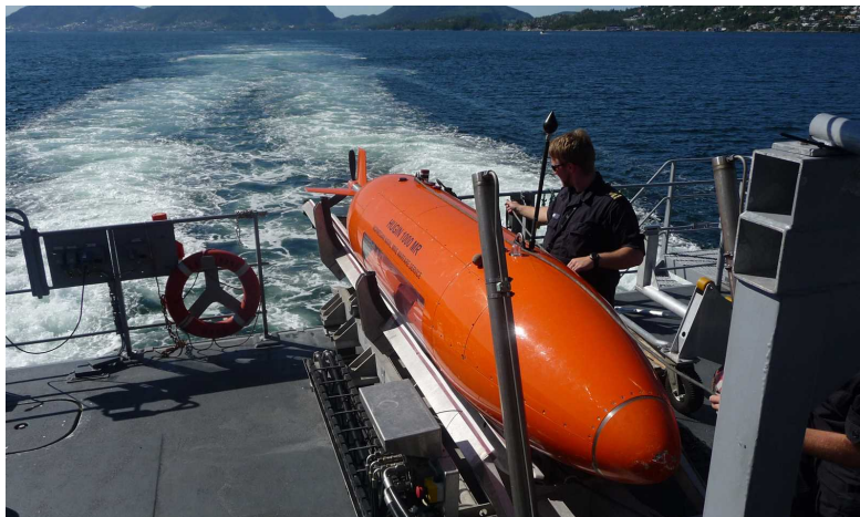
Figure 3: Hugin 1000 AUV on the ship deck before deployment (Courtesy of Kongsberg Maritime)
