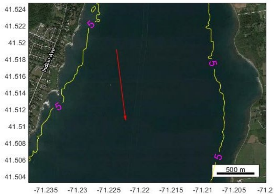
Figure 33: Sakonnet River GPS track line and direction of drift from range testing (06/23/21) with bathymetry contours overlaid (meters).
