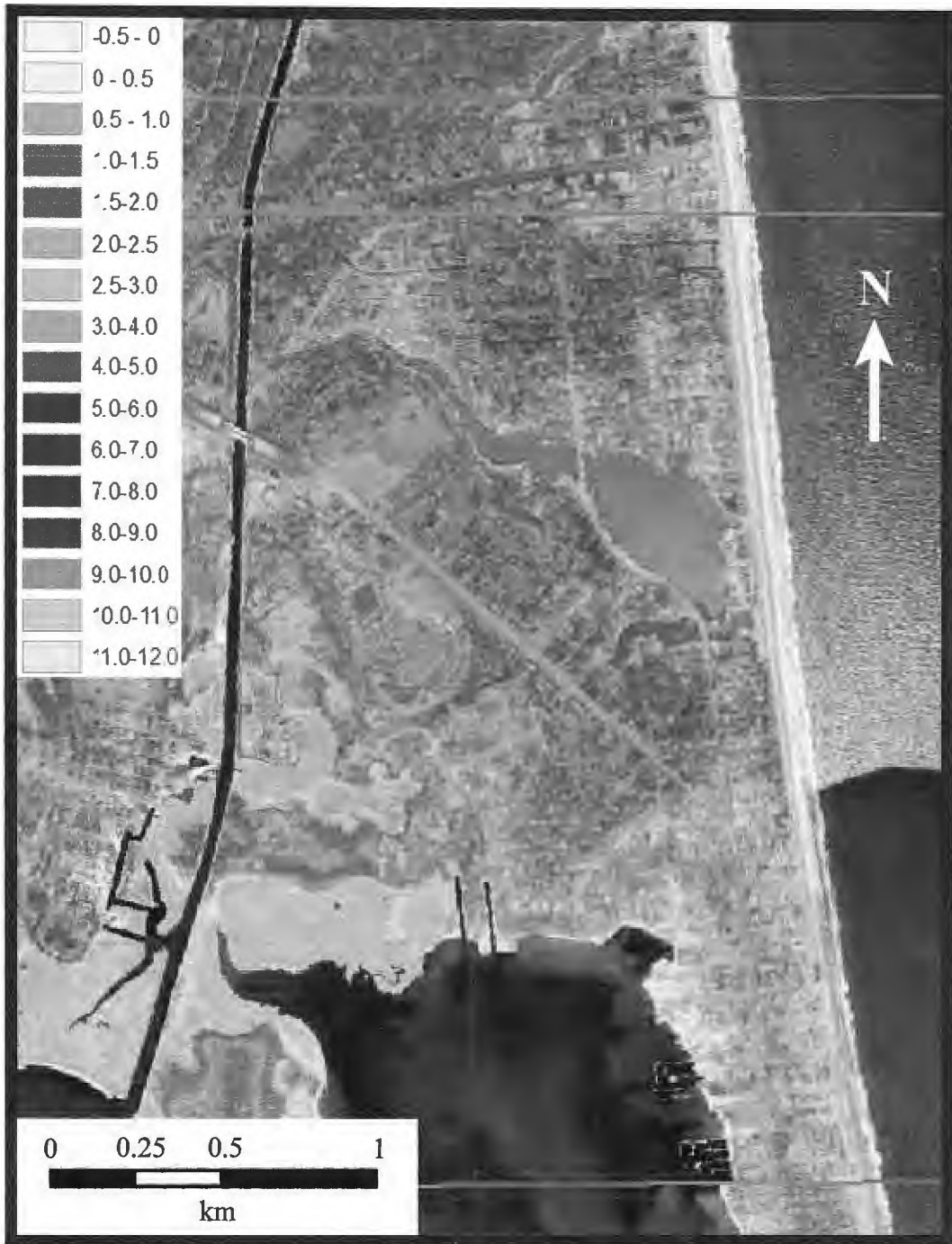
Figure 5. LiDAR elevation map (in meters) of the Rehoboth Beach area. Note that the land surrounding Silver Lake is higher than that surrounding Rehoboth Bay further south. This higher elevation is a result of Silver Lake's location on the Rehoboth headland composed of the more resistant Scotts Corners Formation. Adapted from McCarty, 2009 (Vertical Reference: NAVD88).
