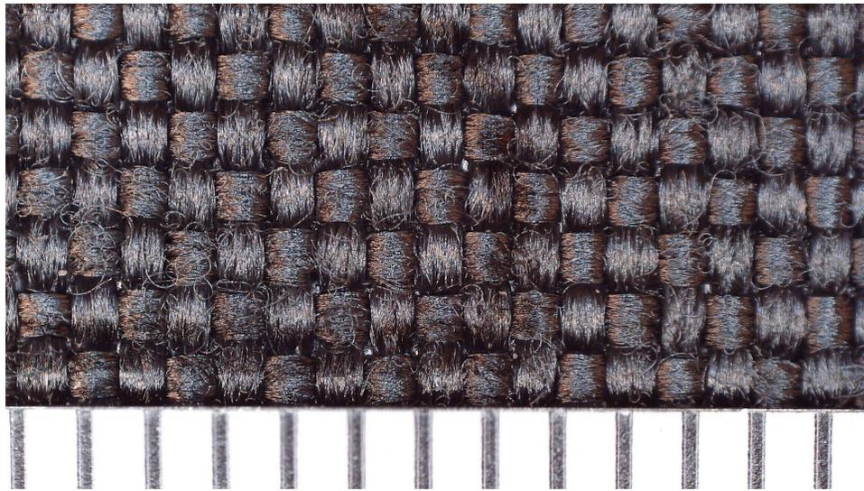
Figure 35: Thread spacing measurement
