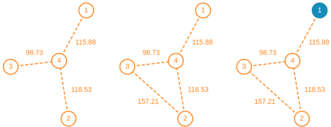
(i) Start with minimum spanning tree (ii) Add minimum-matching edges (3-2 and 1-4) (iii) Start building tour with 1, following Euler Cycle
