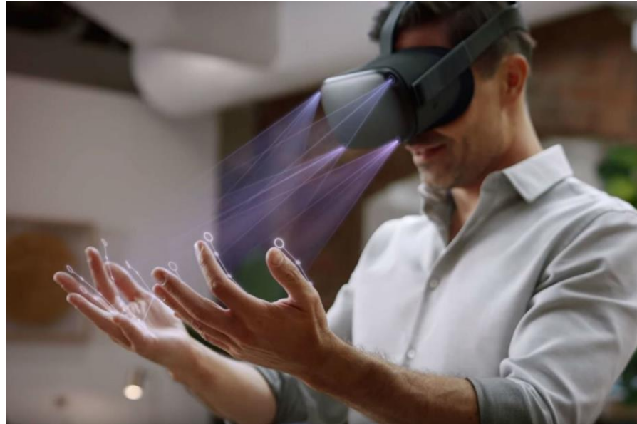
Figure 5: Oculus Quest 2 hand tracking with 4 fish-eye cameras [21]
