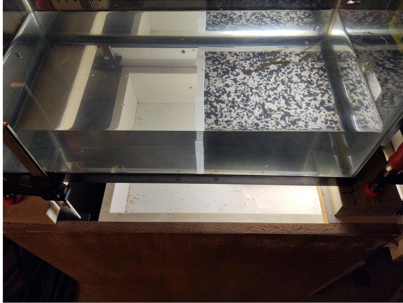
*Figure 5.1: Image of the tank lit from below so as to avoid any glare on the free surface.*
