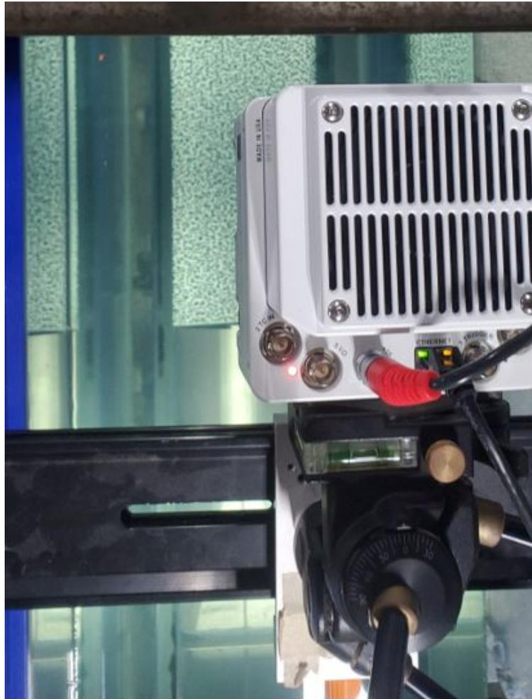
*Figure 5.23: The experimental setup camera's view from above the tank of the speckle pattern mounted underneath the flow channel.*
