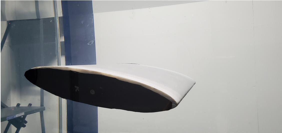
*Figure 4.9: Mounting system for the HDPE foil by itself.*
