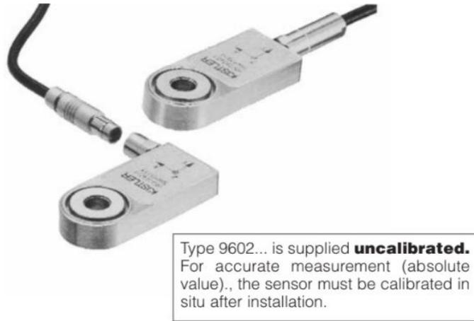
*Figure 4.1: Image of the Kistler type 9602 6-axis piezoelectric force sensor (Kistler, 2016).*
