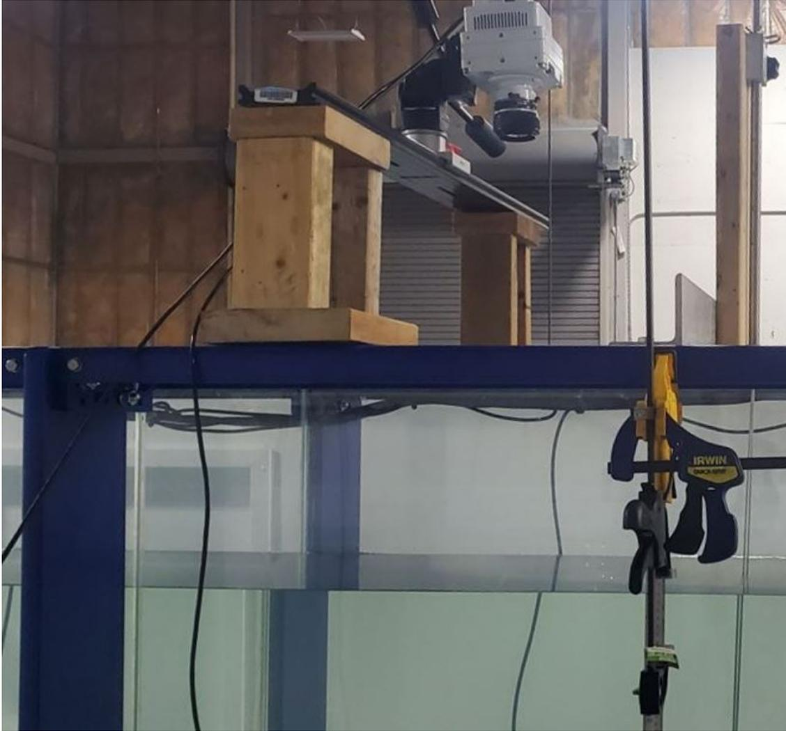
*Figure 5.22: The experimental setup of the camera over the flow channel.*
