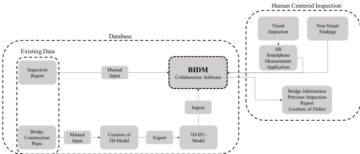
Figure 16: Concept and Dataflow of developed Method (own figure)
