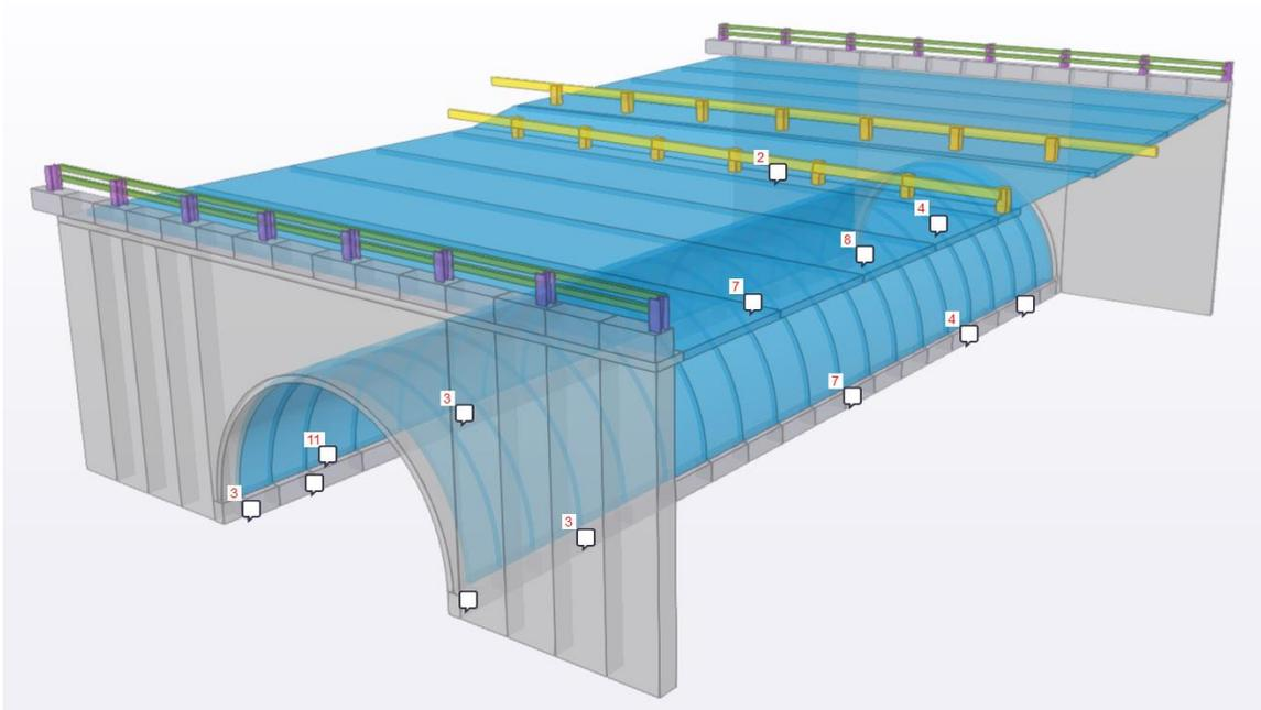
**Figure 31: Jamestown Arch III, Model Overview with Defect Tags' Location, View to North-West (own figure)**
