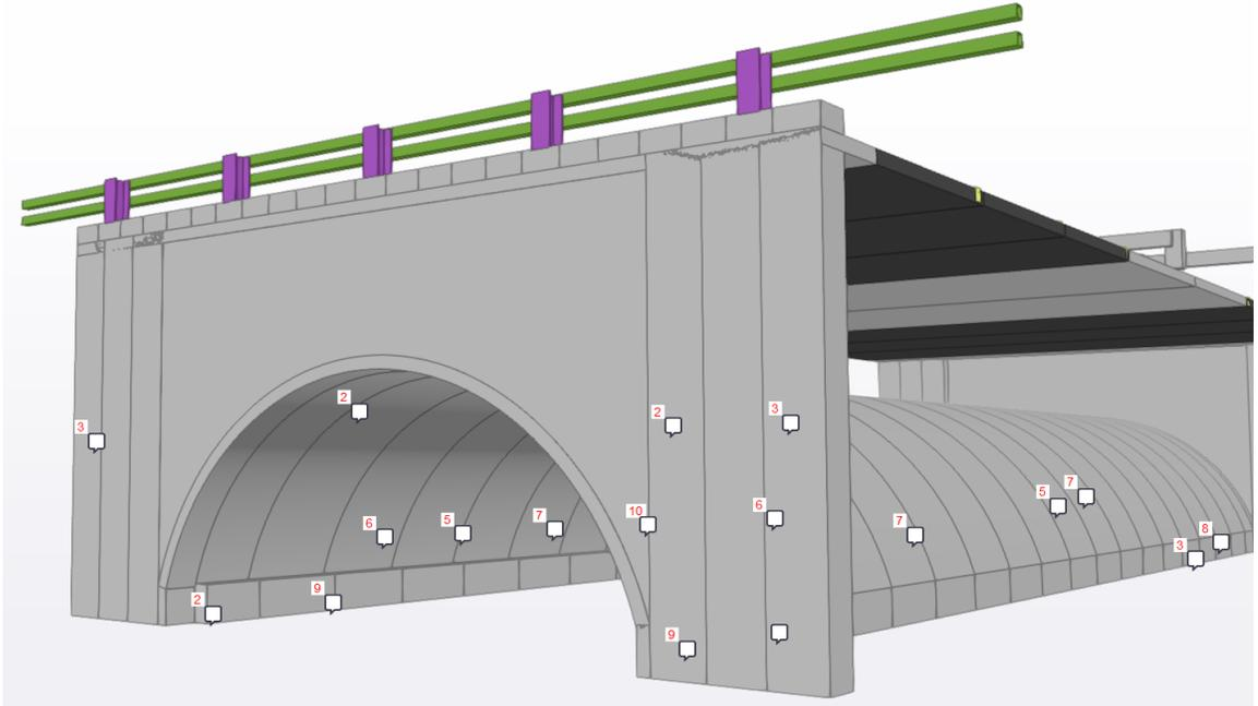
Figure 55: Arch IV View at North Portal to East, Trimble Connect Model View with Defect Tags (own image)
