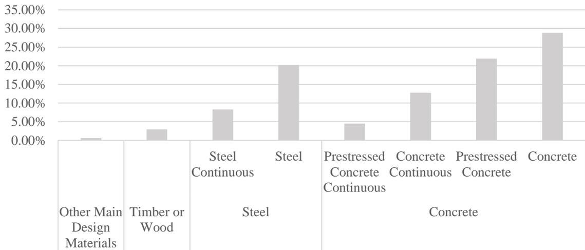
**Figure 17: Share of Main Design Material of US Bridges** (own figure, data: (FHWA, 2020))
