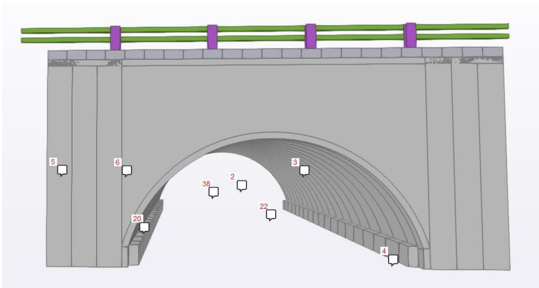
Figure 58: Arch IV View South to North, Trimble Connect Model View with Defect Tags (own image)
