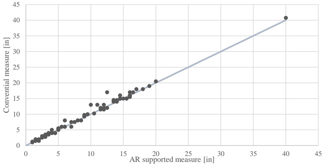
**Figure 36: Sample 1 AR-supported Measures Compared to Conventional Measures** (own figure, own data)
