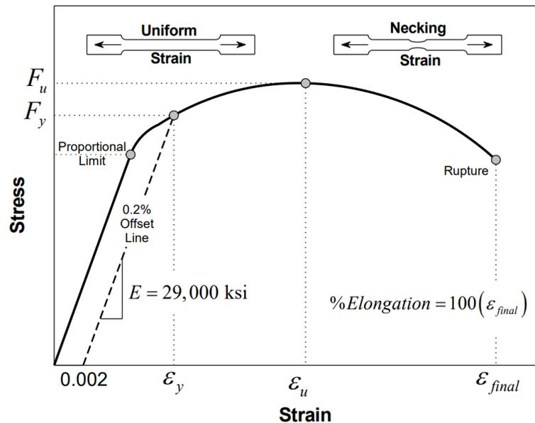
Figure 12: Stress-Strain Curve of regular Construction Steel (Wright, 2015)
