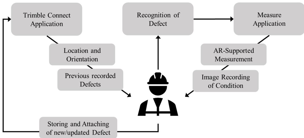
**Figure 25: Human Centered Inspection using Trimble Connect and Measure** (own figure)
