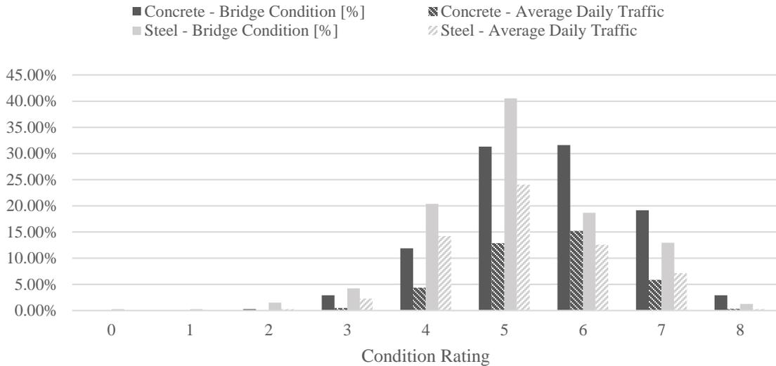
**Figure 20: Correlation of Condition Rating, Material Type and Average Daily Traffic, RI** (own figure, data: (FHWA, 2020))
