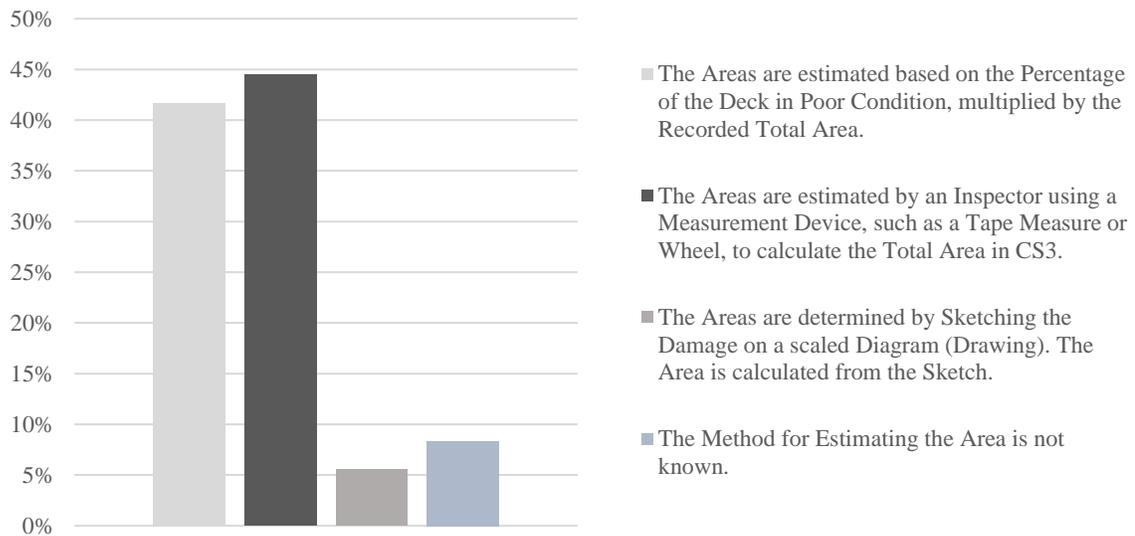
**Figure 3: State DOTs Estimation Method for Deck Element's CS** (own figure, data: (Washer et al., 2019))
