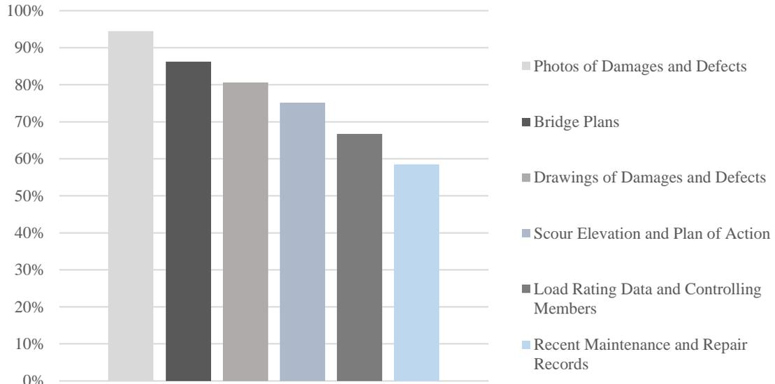
**Figure 4: Additional Information accessible prior to the Inspection** (own figure, data: (Washer et al., 2019))
