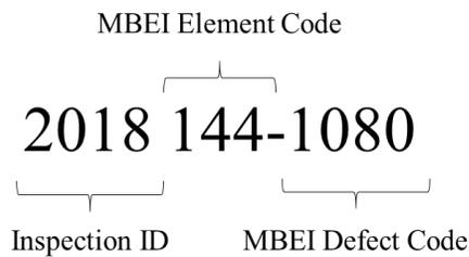
**Figure 28: BIDM Coding Example for Element Defects** (own figure)
