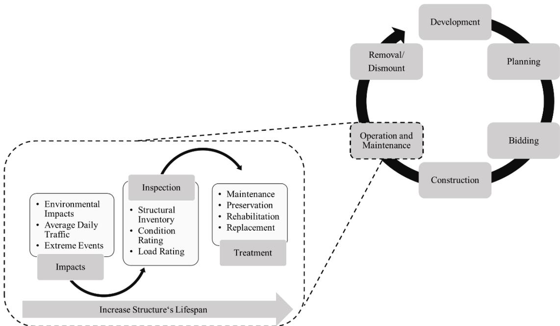
**Figure 1: Bridge Life Cycle Phases with magnified O&M Phase.** (extended and modified (Chipman, Costin, & Yang, 2016))
