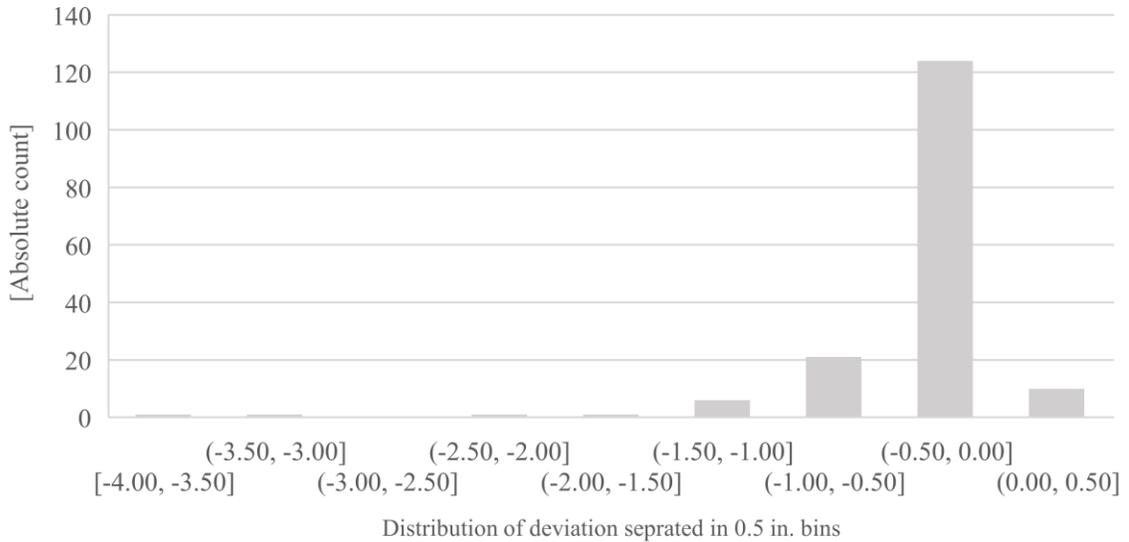
**Figure 38: Sample 1 Histogram of Deviation Distribution** (own figure, own data)
