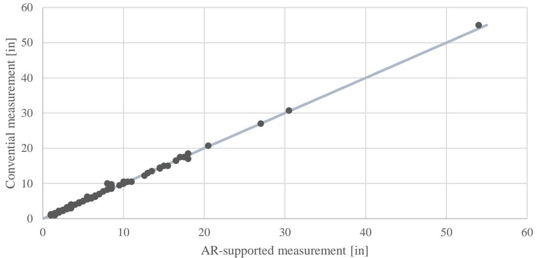
**Figure 39: Sample 2 AR-supported Measures Compared to Conventional Measures** (own figure, own data)
