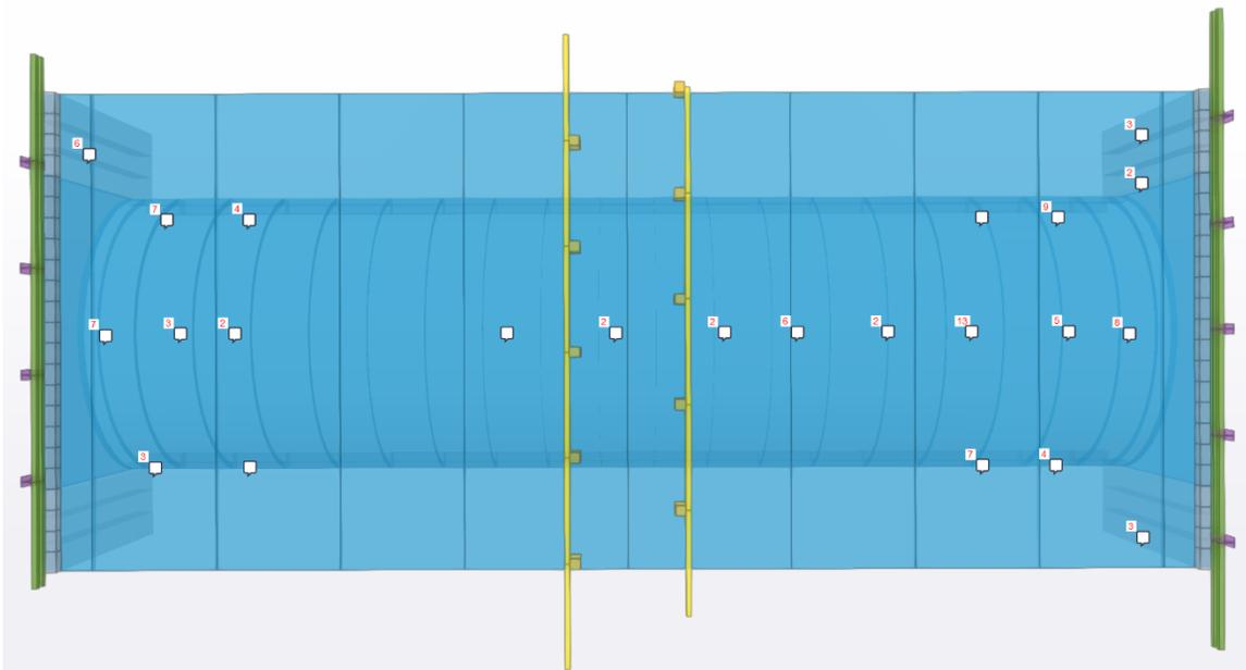
**Figure 35: Arch IV Top View with Defect Tags, Trimble Connect Desktop View (own figure)**
