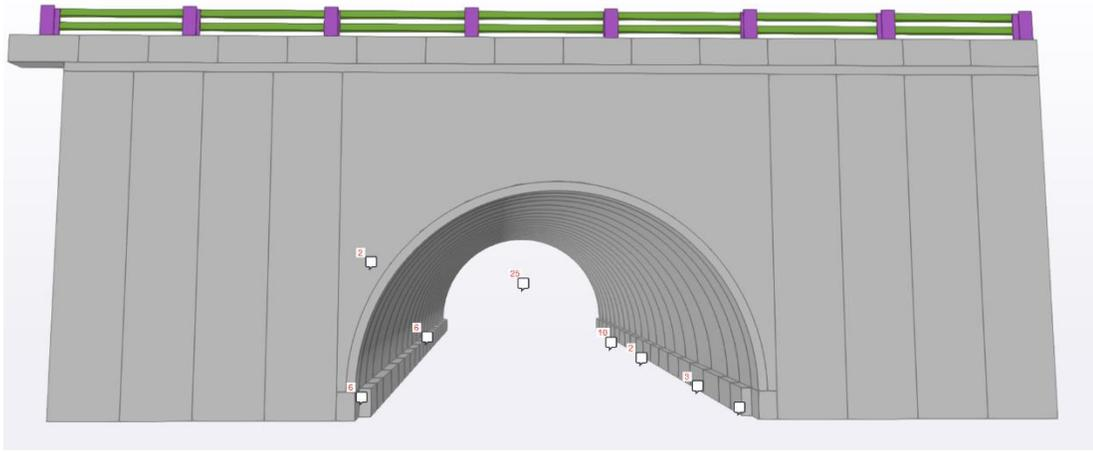
**Figure 52: Arch III View at South Portal to North, Trimble Connect Model View with Defect Tags (own image)**
