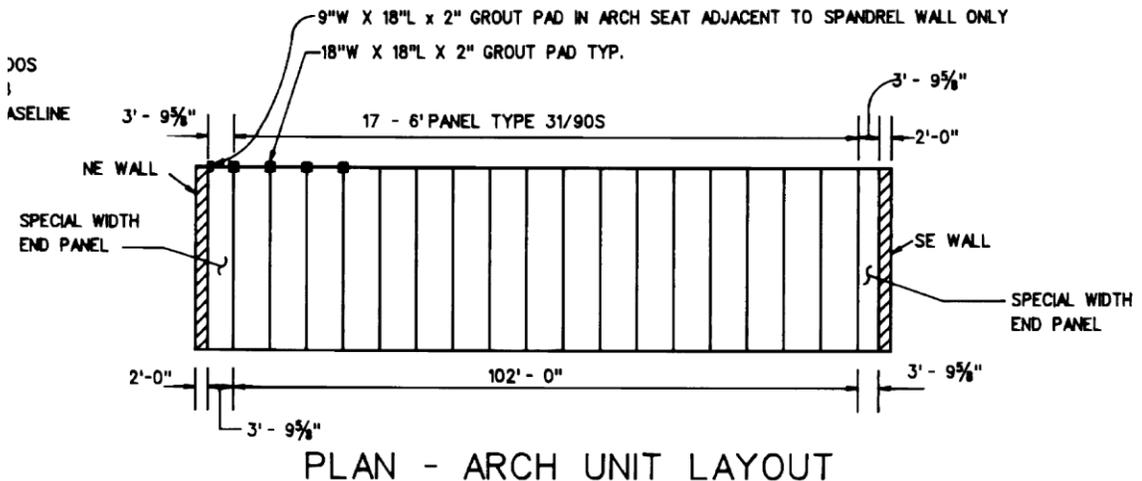
Figure 33: Cut-Out Plan View of Arch IV Construction Plan (cp. Appendix K)
