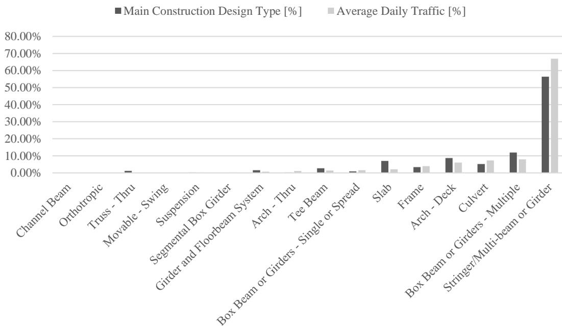
**Figure 21: Correlation of Construction Design Type and Average Daily Traffic, RI** (own figure, data: (FHWA, 2020))
