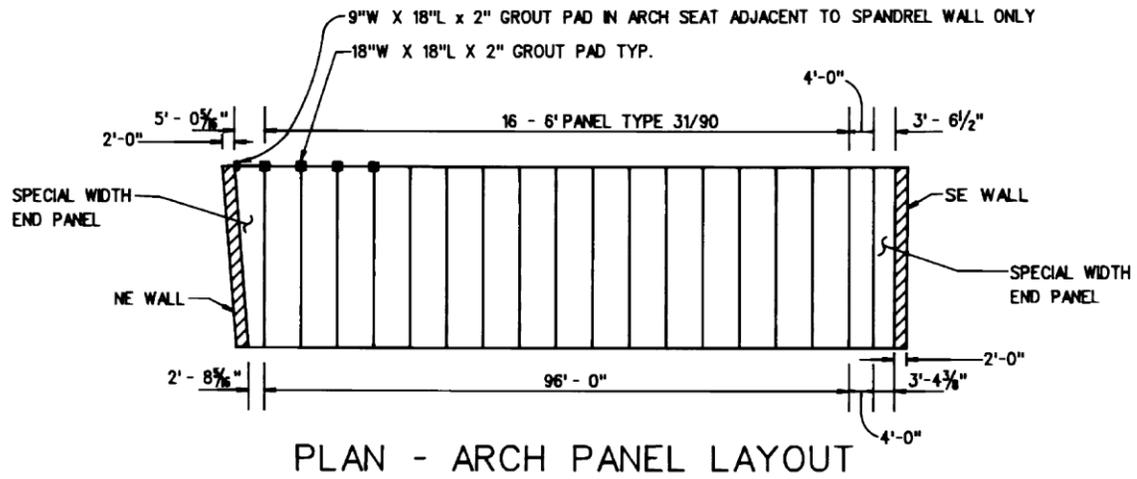
Figure 30: Cut-Out Plan View of Arch III Construction Plan (cp. Appendix I)
