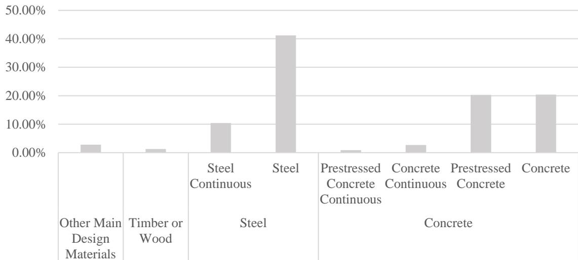
**Figure 18: Share of Main Design Material of Rhode Island Bridges listed in the NBI** (own figure, data: (FHWA, 2020))
