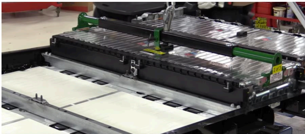
Figure 33: Disassembly step D39, the lifting of four battery modules [21]
