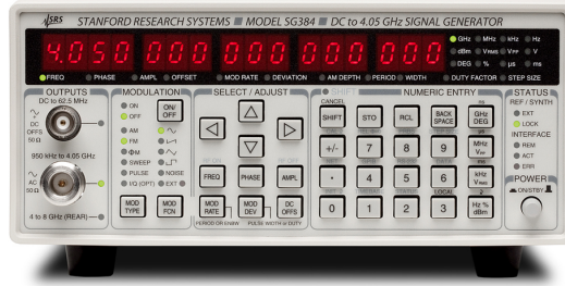
Figure 16: Source generator with rubidium timebase [10].
