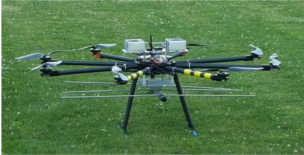
Figure 8: Mounted Yagi Rotation system on Octocopter [15].
