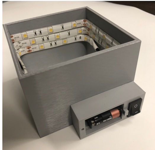
Figure 53. Light Box Electronics
