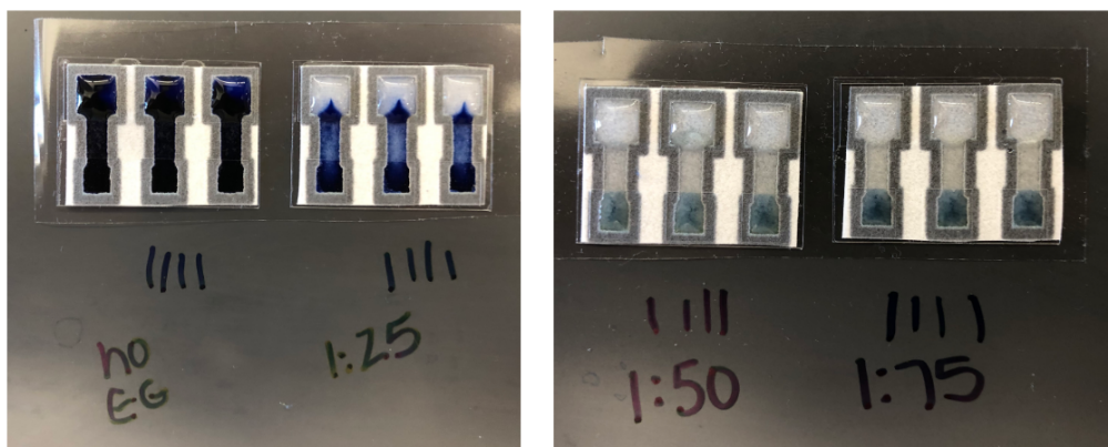
Figure 111. Molybdenum to Ethylene Glycol Ratio Tests
