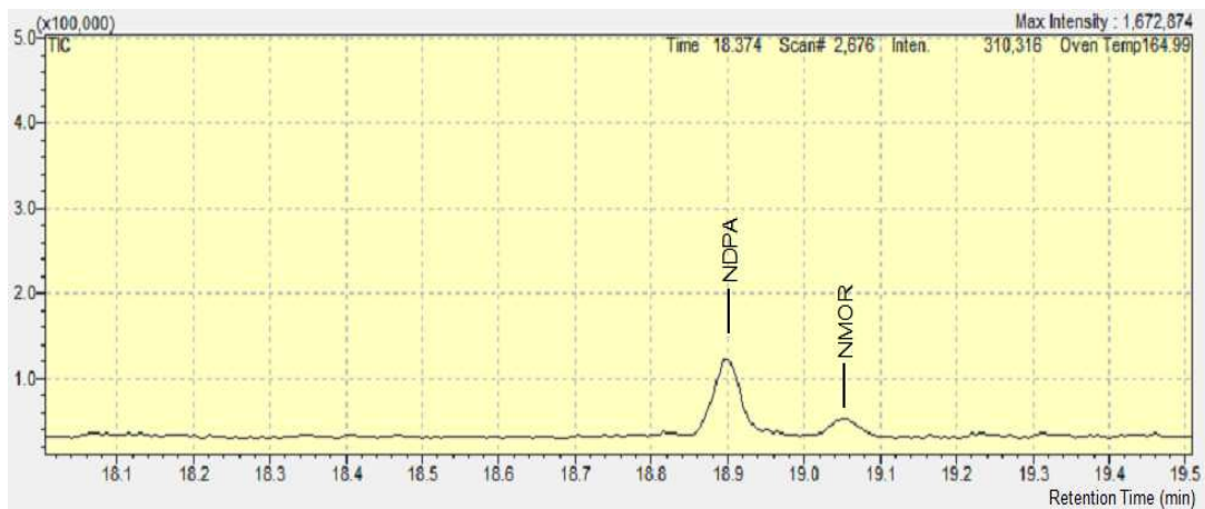
Fig. A3. Magnified view of NDPA and NMOR (2 \mu\text{g/L} ). Low NMOR peak signal suggests 2 \mu\text{g/L} is possible LOD for this target analyte.
