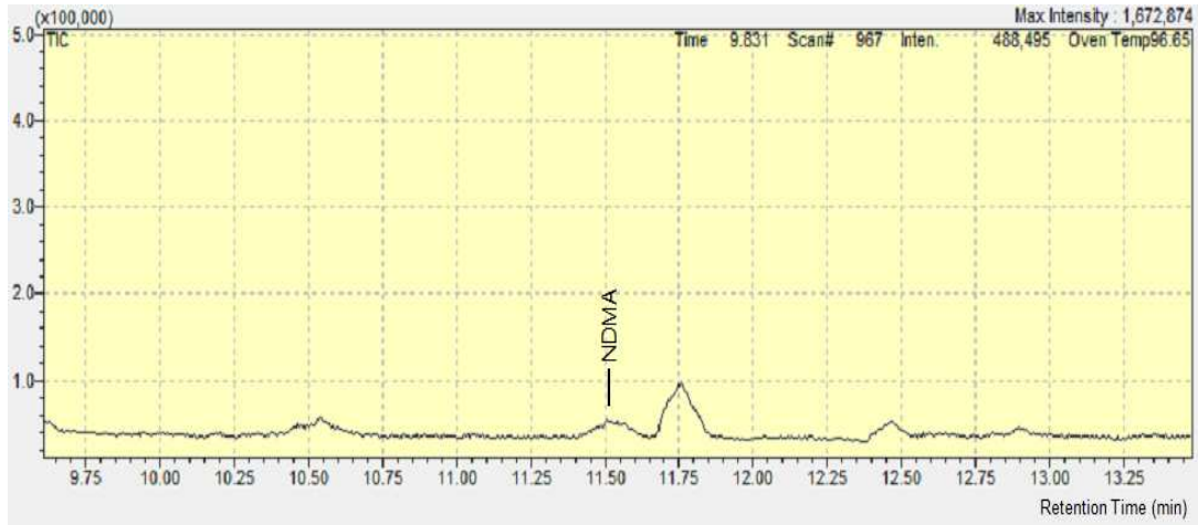
Fig. A1. Magnified view of NDMA (2 \mu\text{g/L} ). The peak at 11.75 min was identified as benzene.
