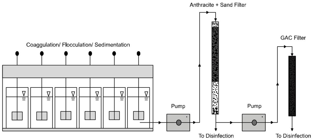
**Figure 2.** Flow-scheme of benchtop water treatment system.
