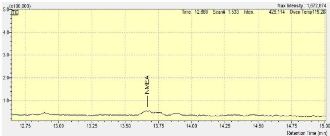
Fig. A2. Magnified view of NMEA (2 \mu\text{g/L} ). Very low peak signal suggests 2 \mu\text{g/L} is possible MDL for this target analyte.
