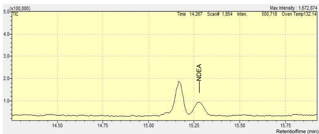
Fig. 2. Magnified chromatogram showing poor separation between NDEA and an identified hydrocarbon.
