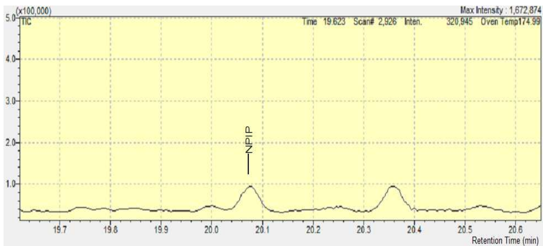
Fig. A4. Magnified view of NPIP (2 \mu\text{g/L} ). The peak at 20.36 min was identified as a hydrocarbon.
