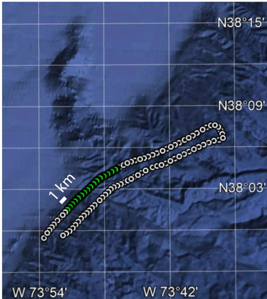
Figure 23. Wire Flyer survey waypoints overlaid on Google Earth bathymetry. The major portion of the observed shallow water front is indicated by the green waypoints
