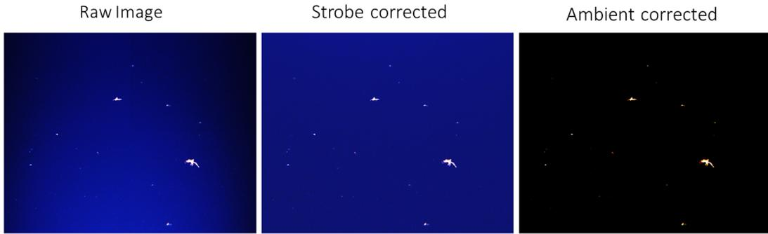
Figure .35. Results of the two step image lighting normalization. A) Raw image from the color camera in the stereo pair. B) Flattened image data after subtracting the signed strobe lighting representation. C) Foreground isolated image data after subtracting the calculated ambient background lighting.
