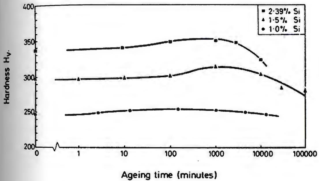
Figure 3-8: Effects of silicon content on the aging characteristics of binary Ti-Si alloys at 550°C (from reference [45]).
