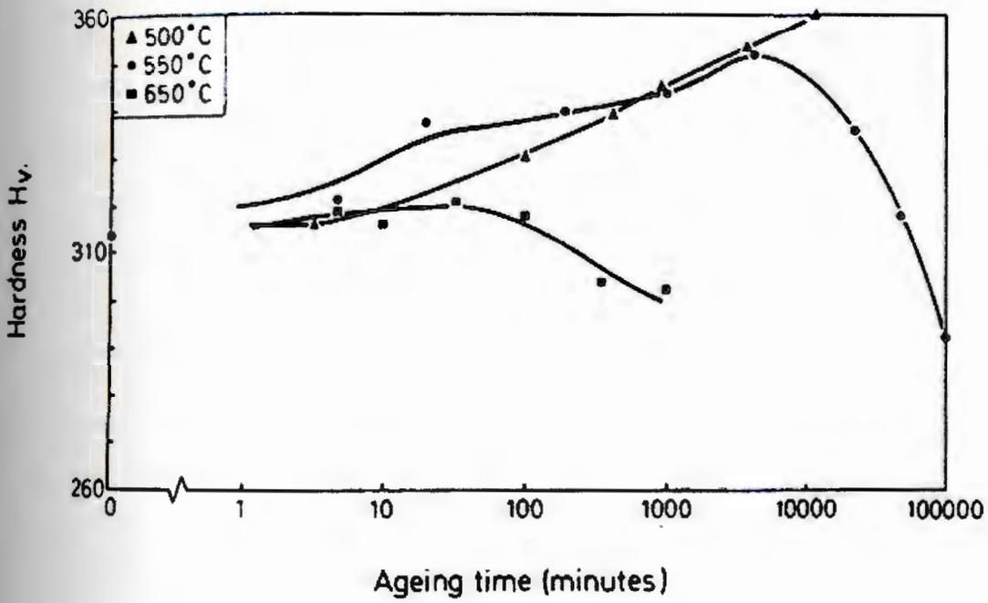
Figure 3-7: Effects of temperature on the aging characteristics of Ti-5%Zr-1%Si (from reference [45]).
