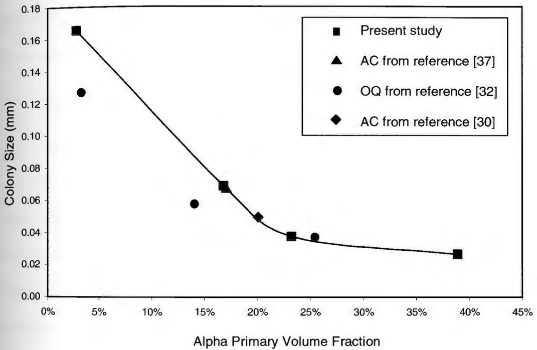
Figure 2-18: Colony size measurements from selected water-quenched specimens and from literature for IMI 834.
