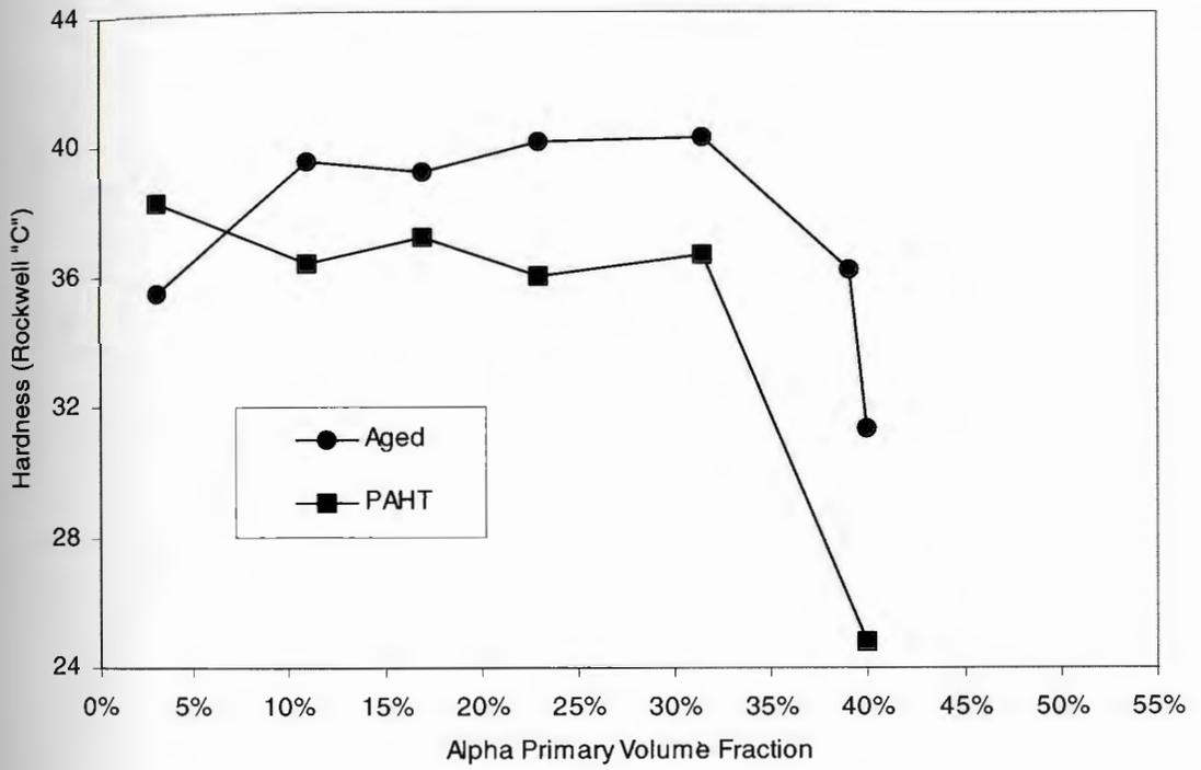
Figure 2-22: Effect of  $\alpha_2$  removal on hardness  $R_C$  in IMI 834.
