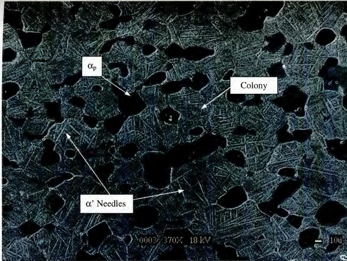
Figure 2-6: Microstructure of IMI 834 (heat-treated and aged to 23%  $\alpha_p$  volume fraction).
