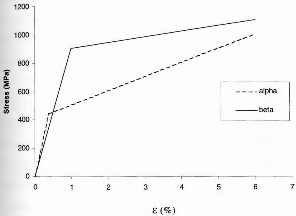
Figure 2-21: Stress-strain curves for  $\alpha$  and  $\beta$  (from ref. [54]).
