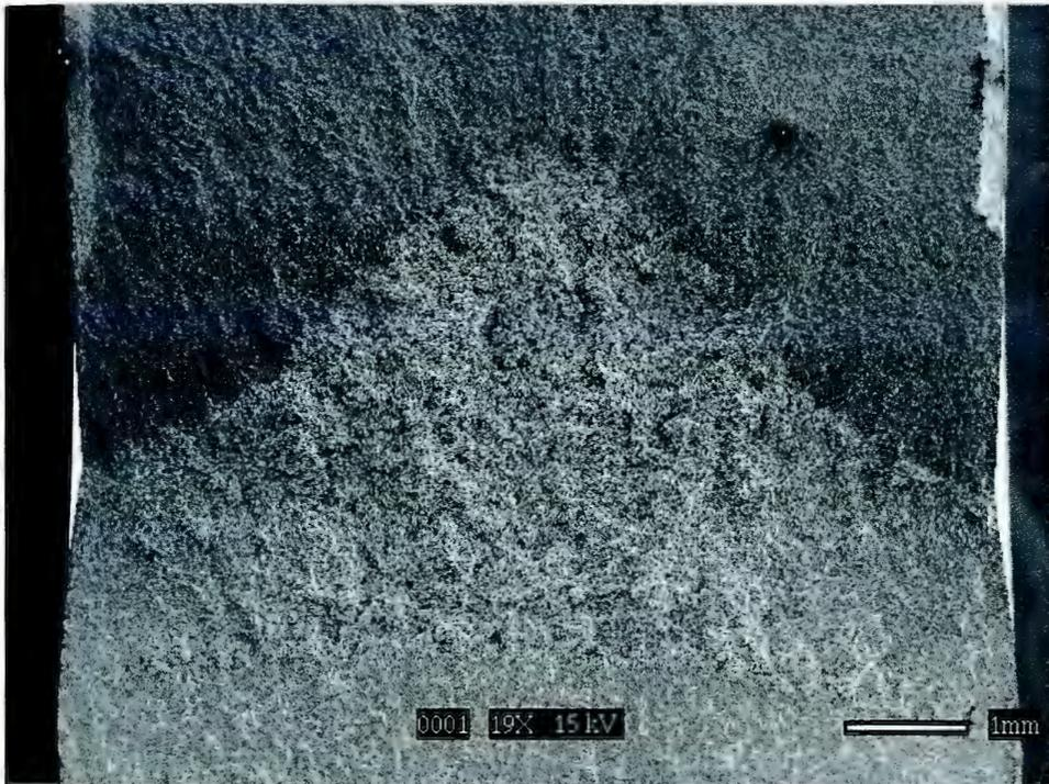
*Figure 4-10: Fracture surface showing the transition between test conditions 0.05 Hz and 0.003 Hz as well as between 0.003 Hz and failure on the 20%  $\alpha_p$  vf specimen.*
