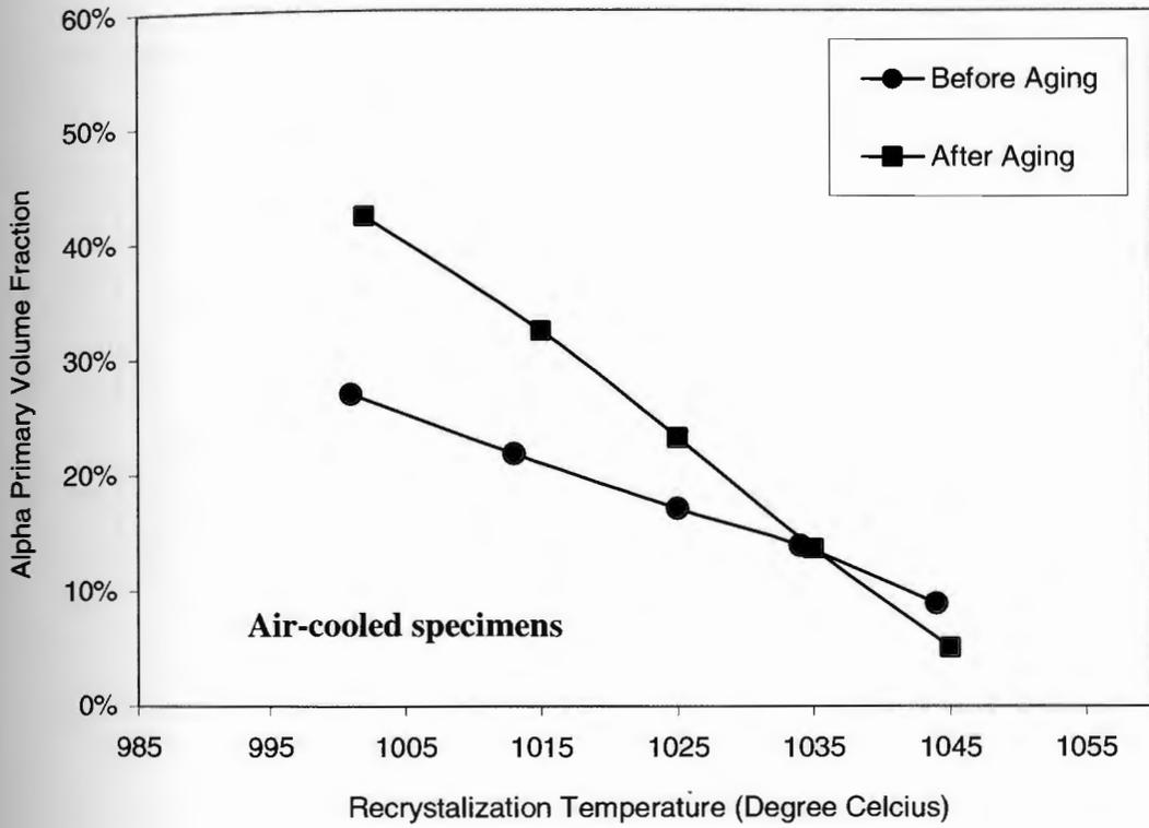
Figure 2-16: Effects of aging on the  $\alpha_p$  volume fraction for air-cooled specimens of IMI 834.
