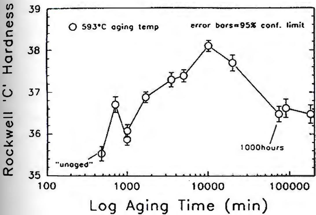
Figure 3-11: Effects of aging on air-cooled Ti-1100 heat treated at 1093°C and "stabilized" at 593°C for 8-hours (from ref. [49]).
