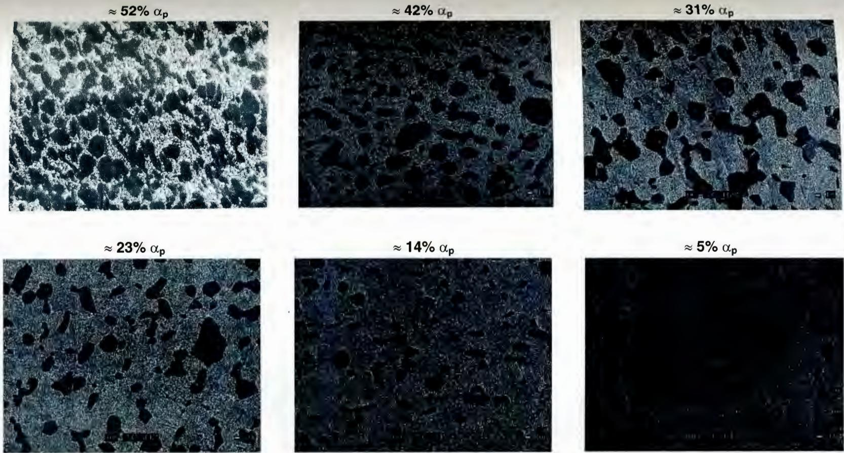
Figure 2-15: Air-cooled IMI 834 microstructures.
