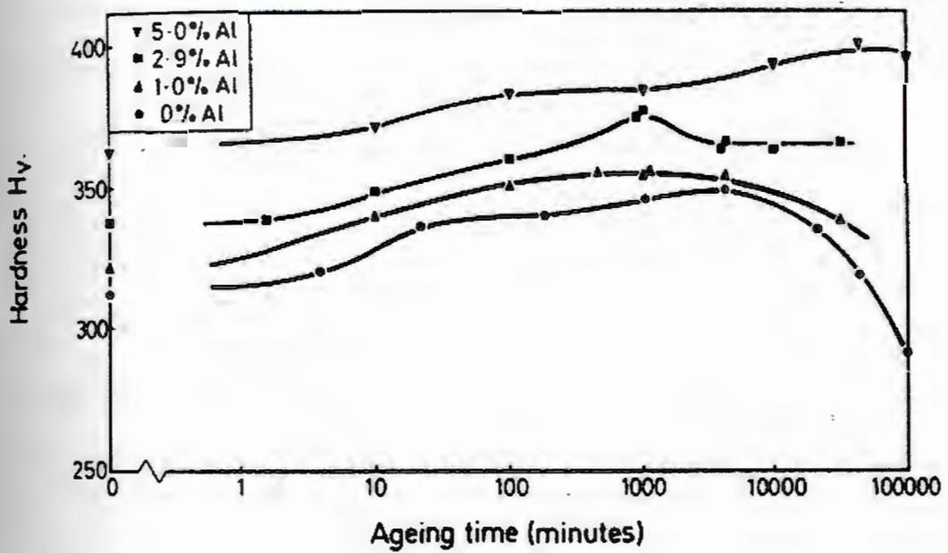
Figure 3-10: Effects of aluminum content on the aging characteristics of the quaternary Ti-5%Zr-1%Si-Al alloy at 550°C (from reference [45]).
