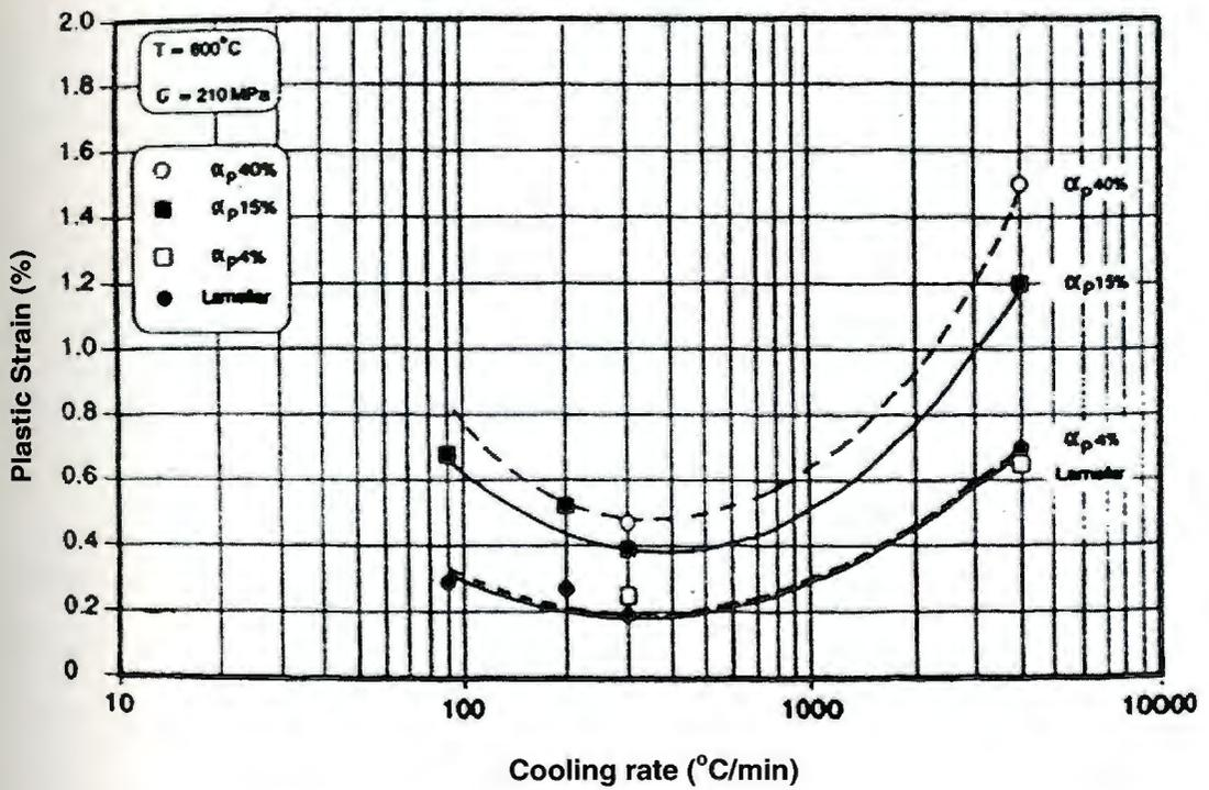
Figure 2-11: Effect of cooling rate on creep strain of near- $\alpha$  titanium alloy IMI 834 (from ref. [13])
