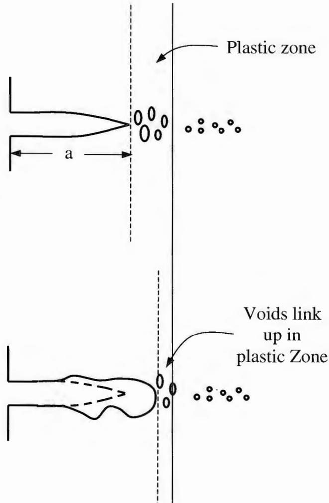
Figure A-5: Schematic representation of crack propagation by ductile tearing.
