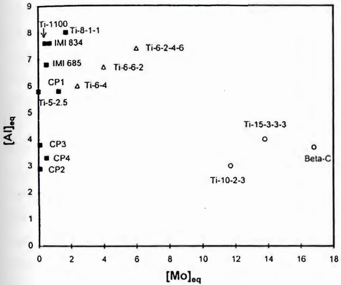
Figure.2-4: Aluminum and molybdenum equivalencies for Titanium Alloys (from ref. [32])
