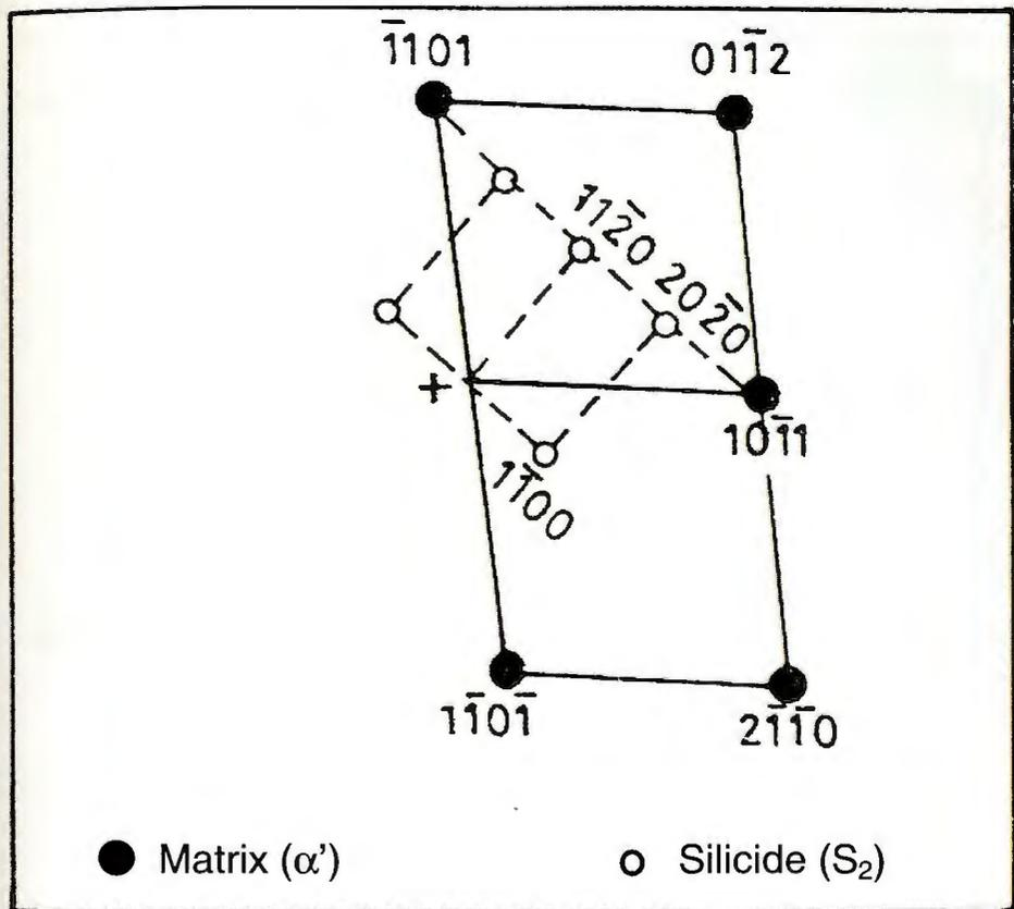
Figure 3-4: Schematic representation of TEM observations of IMI 829 aged for 24-hours at 625°C (from ref. [19]).
