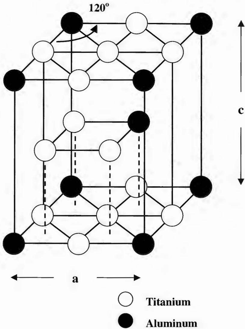
Figure 3-1: Lattice Structure of  $\alpha_2$  ( $Ti_3Al$ ) intermetallic.
