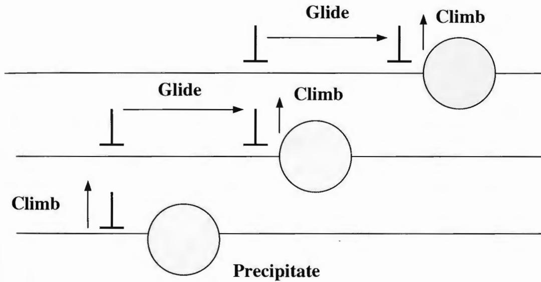
Figure A-3: Schematic representation of creep cause by climb-glide sequence.
