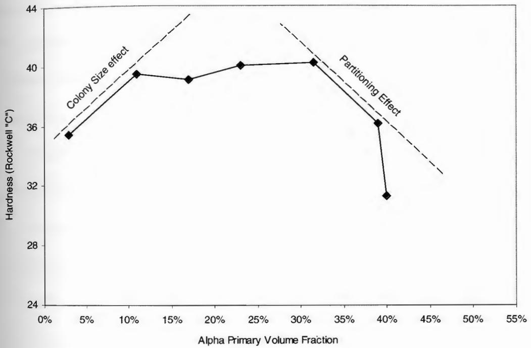
Figure 2-25: Colony size and partitioning element effects for-water-quenched IMI 834 specimens.
