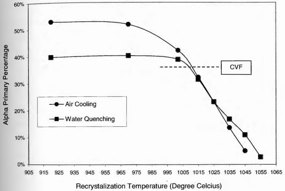
Figure 2-17: Effect of cooling rate on the  $\alpha_p$  volume fraction of IMI 834.
