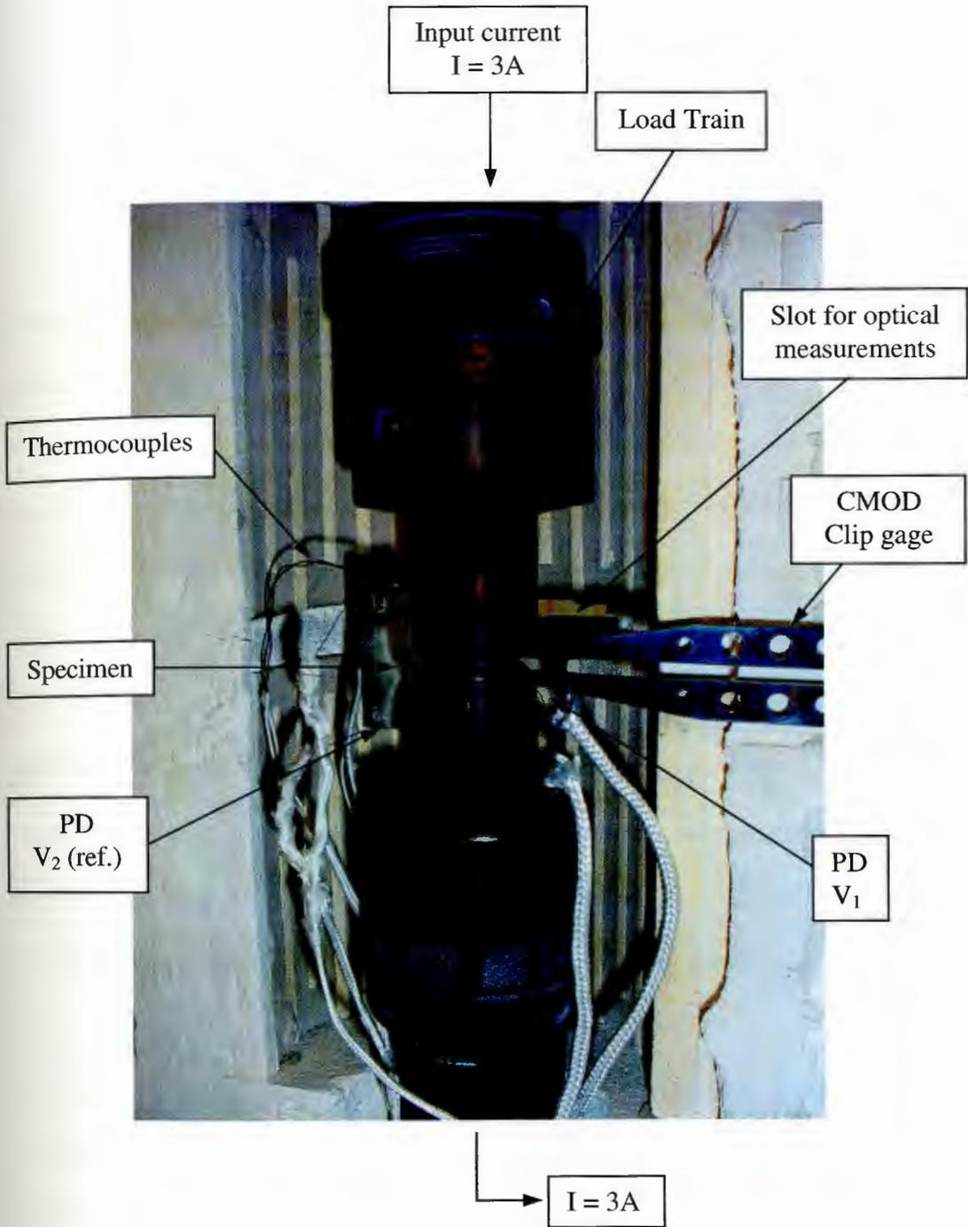
Figure 4-3: Clamshell furnace and loaded specimen with spot-welded thermocouples and Potential Drop (PD) wires.
