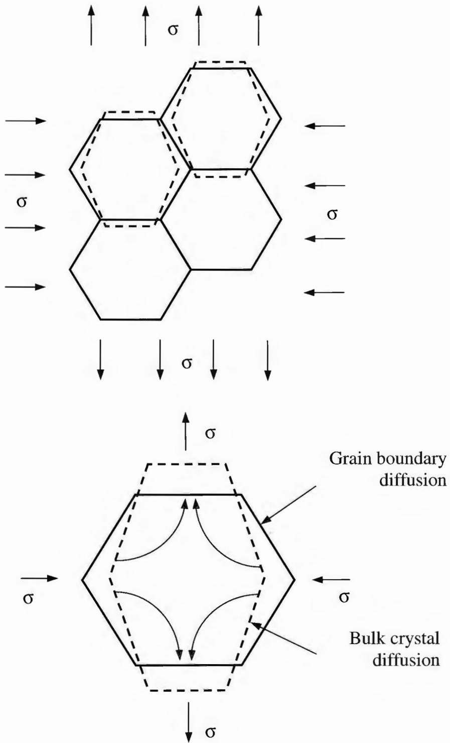
Figure A-4: Schematic representation of diffusion creep.
