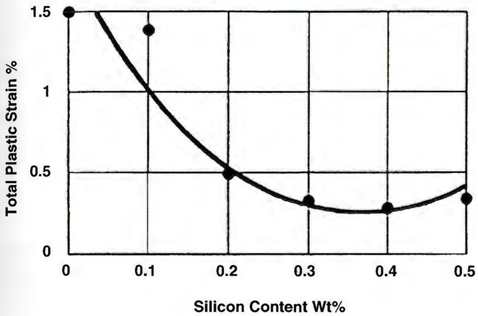
*Figure.2-3: Effect of silicon content on the creep behavior of IMI 834 alloy (from ref. [11]).*
