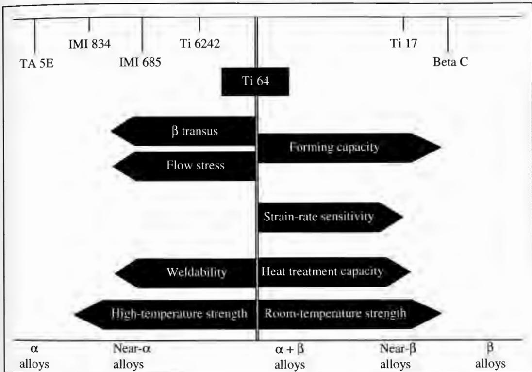
Figure 2-2: Main characteristics of the different titanium alloy families (from ref. [2]).
