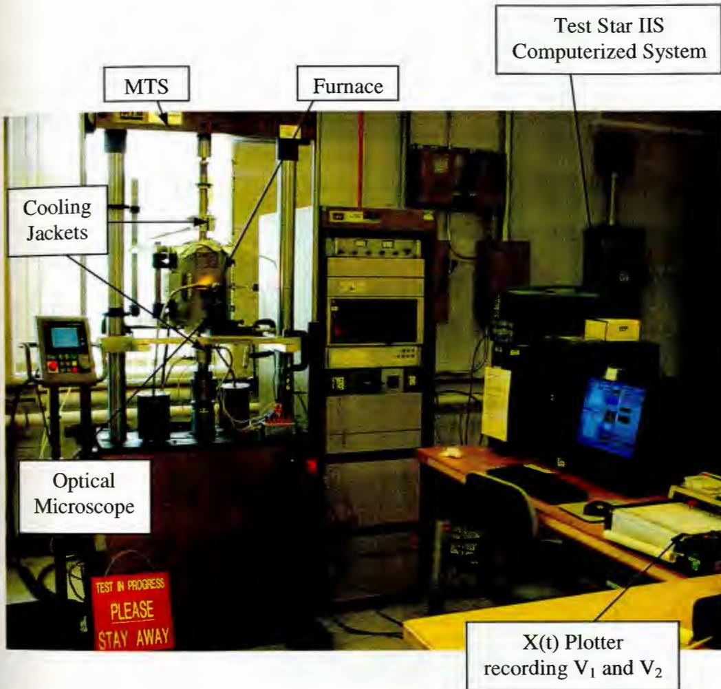
*Figure 4-2: MTS servo-hydraulic material testing system with clamshell furnace controlled by the Test Star IIS computer environment.*
