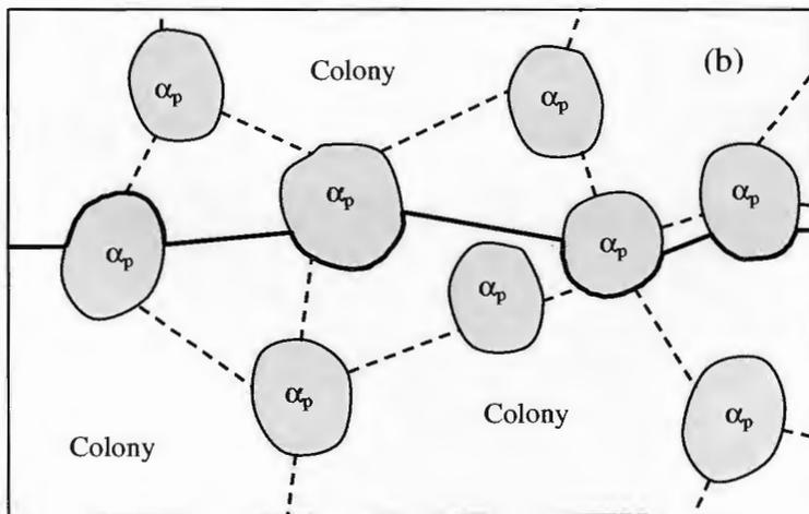
Figure 4-11: Schematic of possible crack path in both  $\alpha/\beta$  colony and primary alpha: (a) trans-colony / trans-alpha particle; (b) trans-colony / inter-alpha boundary.
