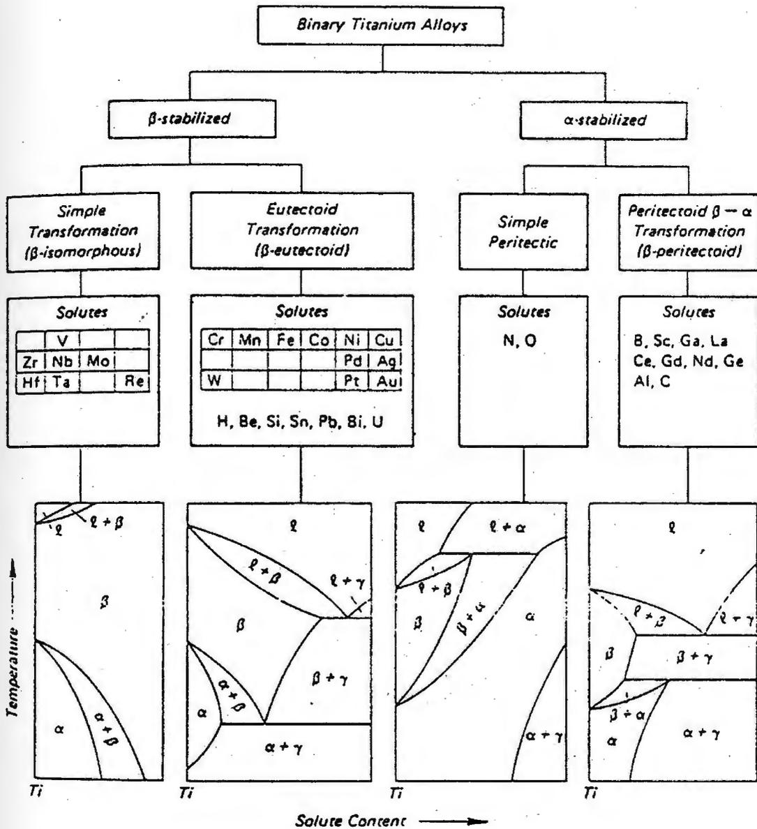
" $\alpha$ " and " $\beta$ " are hcp and bcc solid-solution alloys, respectively, and " $\gamma$ " represents an intermetallic compound.
