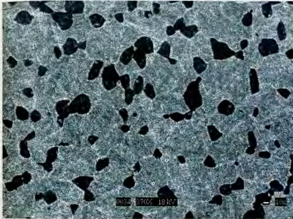
*Figure 4-4: IMI 834 solution treated at 1035°C for 2-hours and water-quenched followed by aging at 700°C for 2-hours (20%  $\alpha_p$  vf).*
