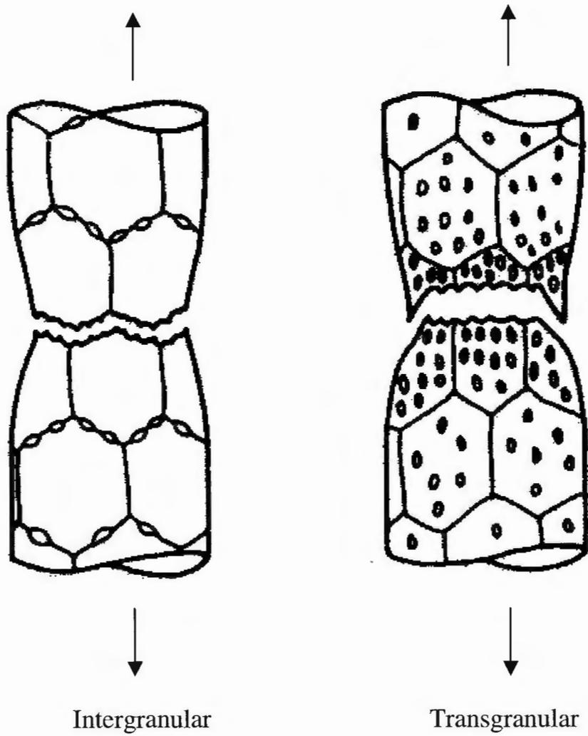
*Figure A-7: Schematic representation of intergranular and transgranular fracture mechanisms.*
