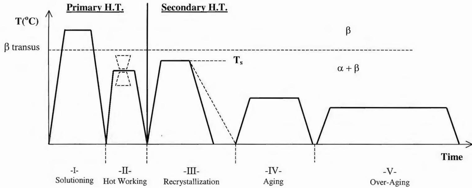
Figure 3-12: Thermal cycle applied in duplex microstructures showing over-aging process.
