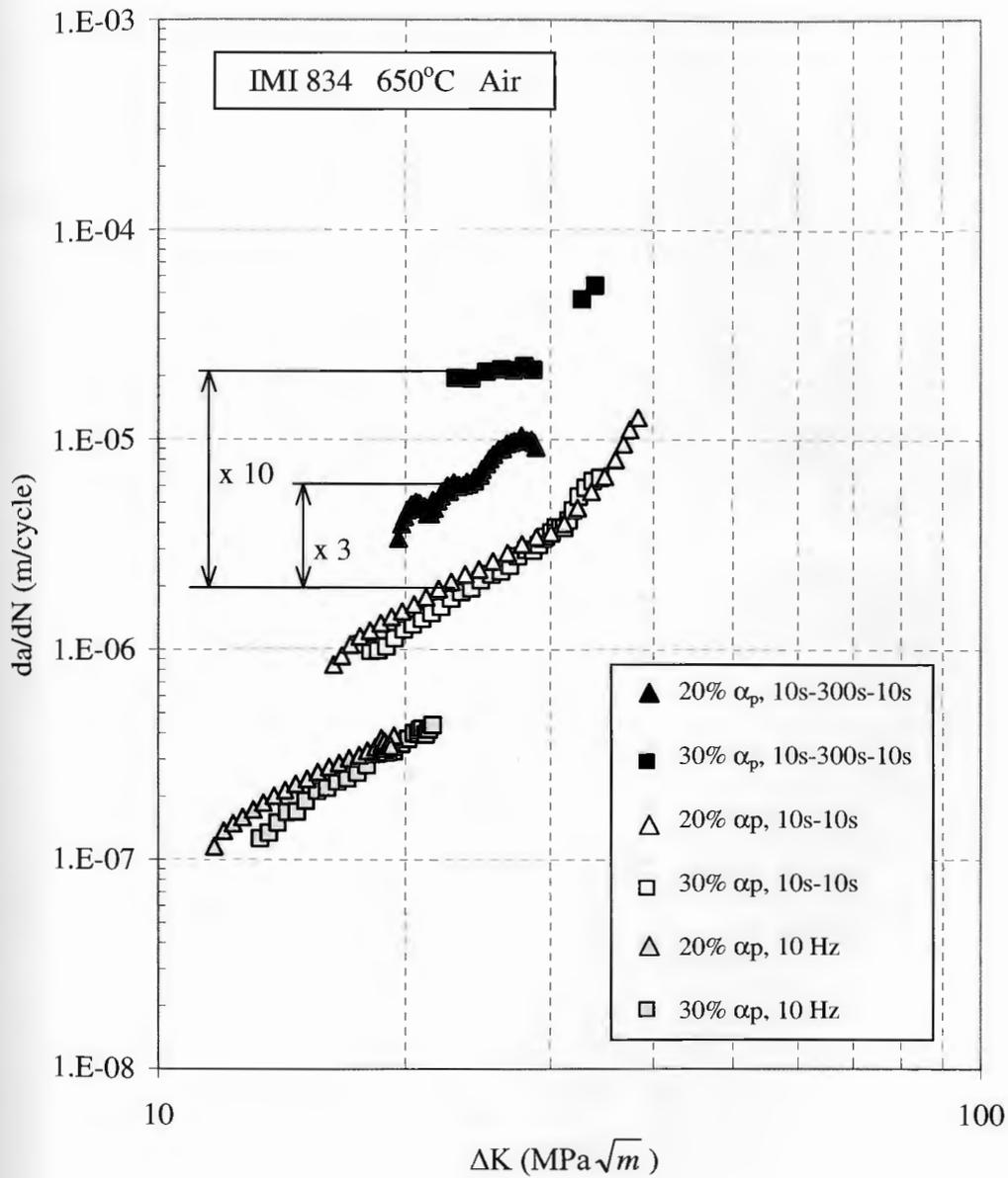
Figure 4-6: Effect of loading frequency and 5 minute hold time at peak stress on Fatigue Crack Growth Rate of IMI 834 at 650°C.
