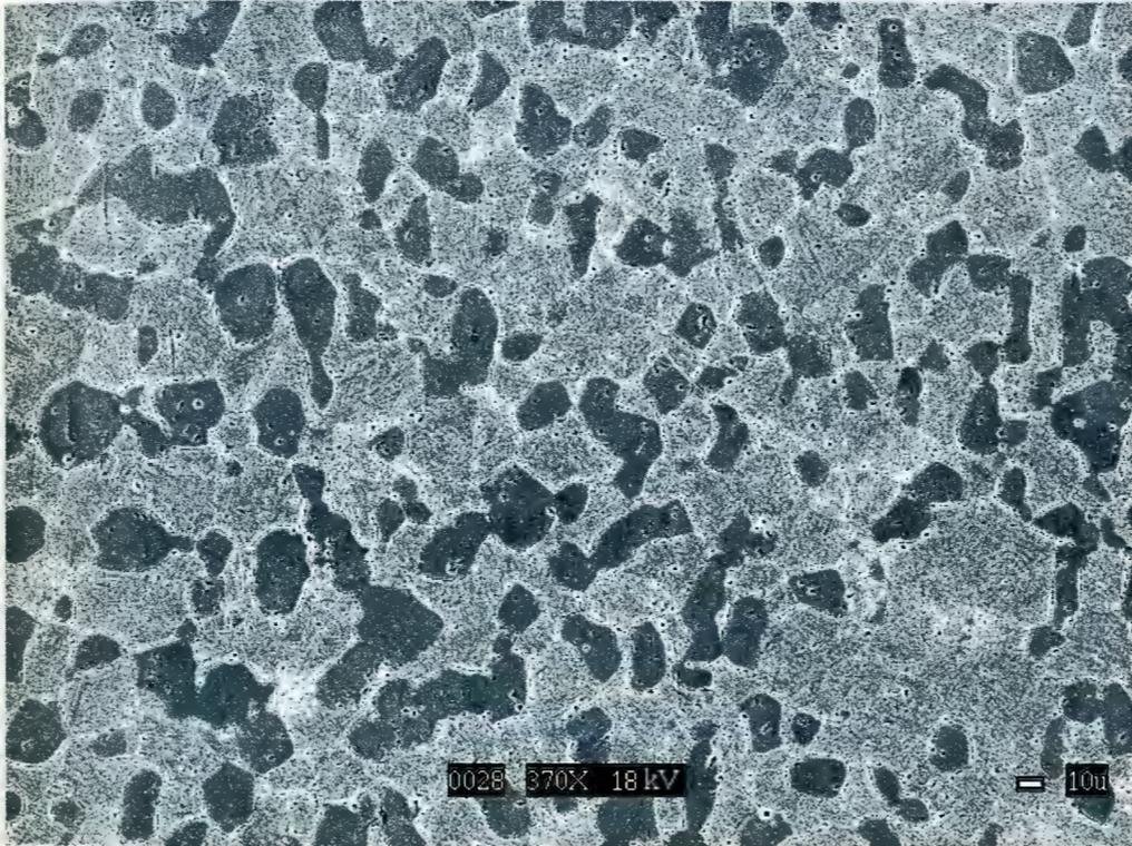
*Figure 4-5: IMI 834 solution treated at 1010°C for 2-hours and water-quenched followed by aging at 700°C for 2-hours (30%  $\alpha_p$  vf).*
