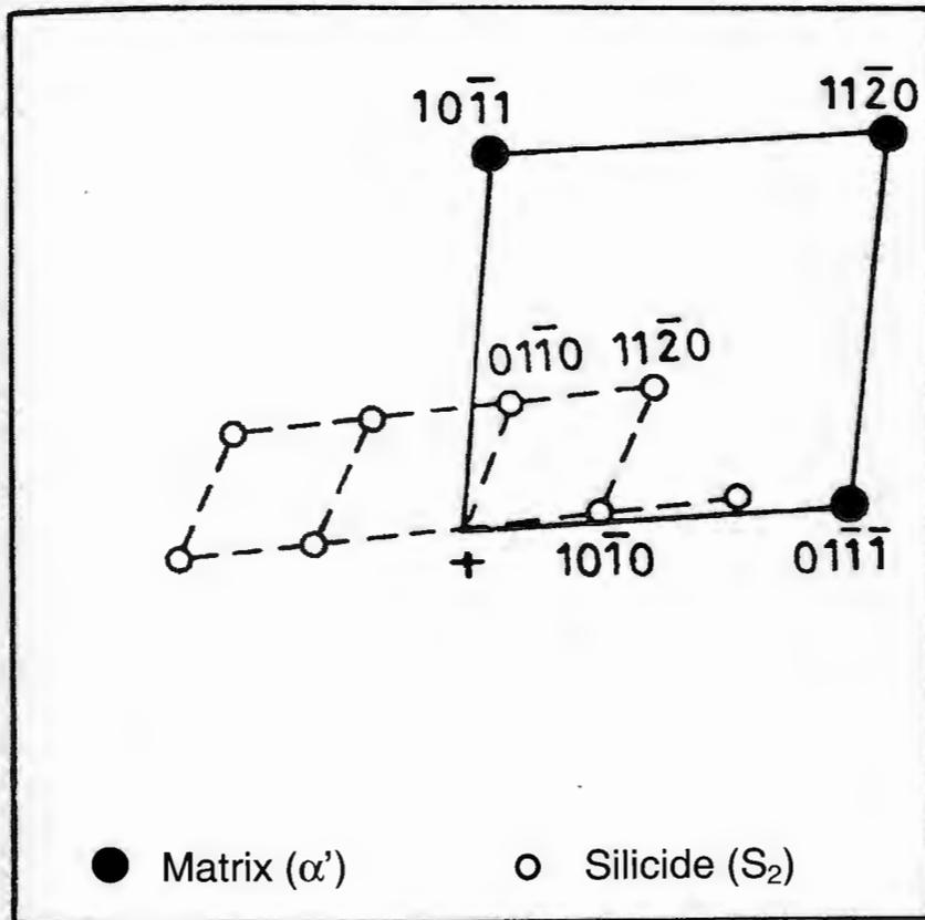
Figure 3-6: Schematic representation of TEM observations of IMI 829 aged for 24-hours at 800°C (from ref. [19]).
