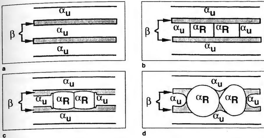
Figure 2-8: Schematic of the mechanism of globularization from lamellar microstructures: (a) unrecrystallized, (b) beginning of recrystallization, (c)  $\alpha_R$  moving into a side plates, (d)  $\alpha_R$  consuming into a side plates (from ref. [51]).
