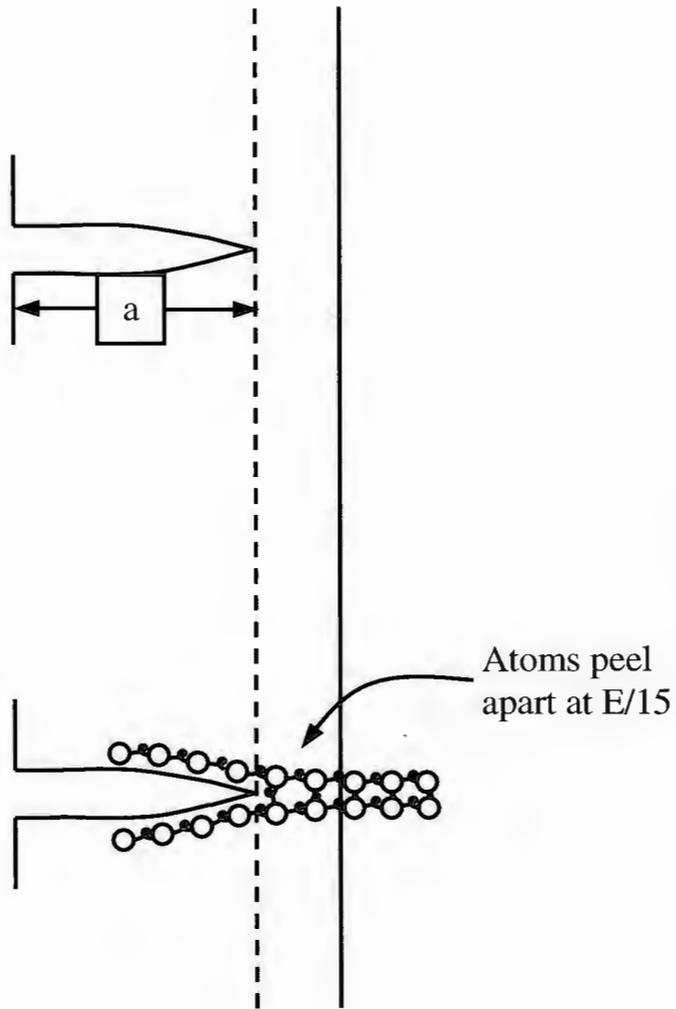
Figure A-6: Schematic representation of crack propagation by cleavage.
