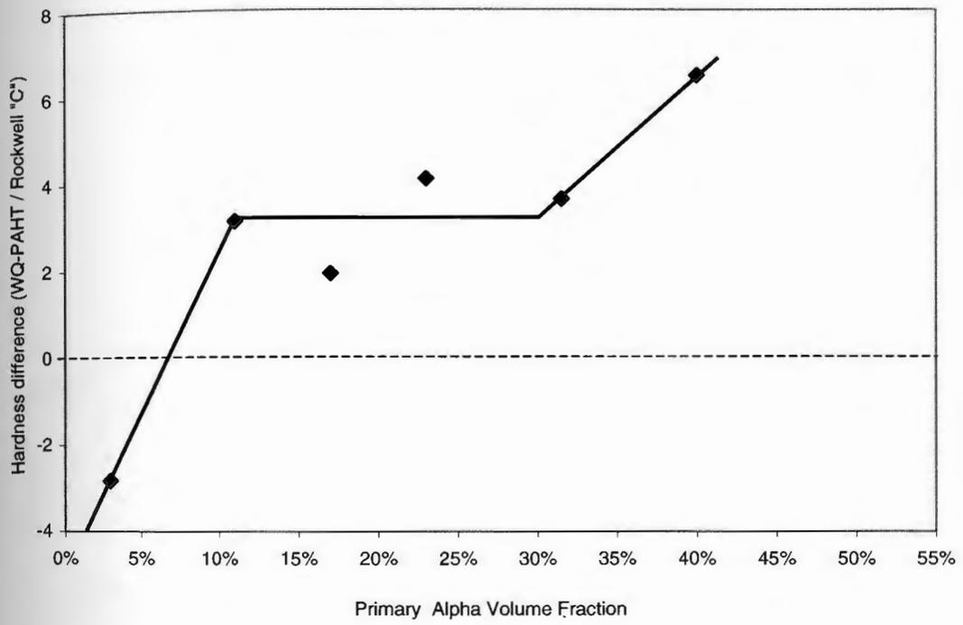
Figure 2-23: Difference of Rockwell "C" hardness results for water-quenched/aged and water-quenched/aged/PAHT IMI 834.
