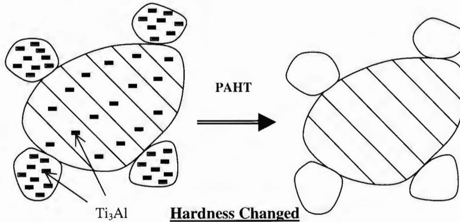
Figure 2-24: Effect of PAHT on hardness of low and high  $\alpha_p$  volume fraction of IMI 834.
