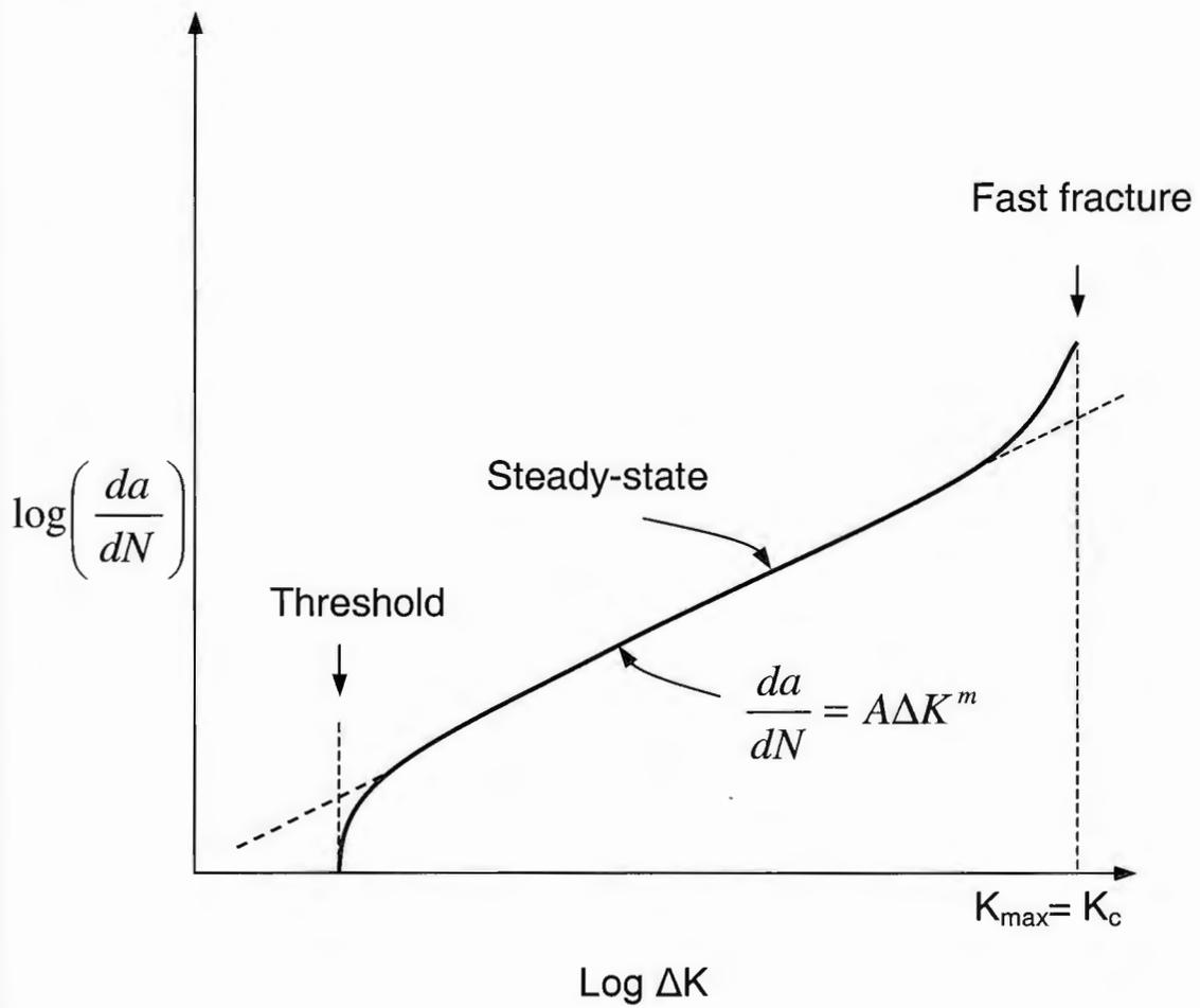
Figure A-2: Typical shape of a fatigue curve
