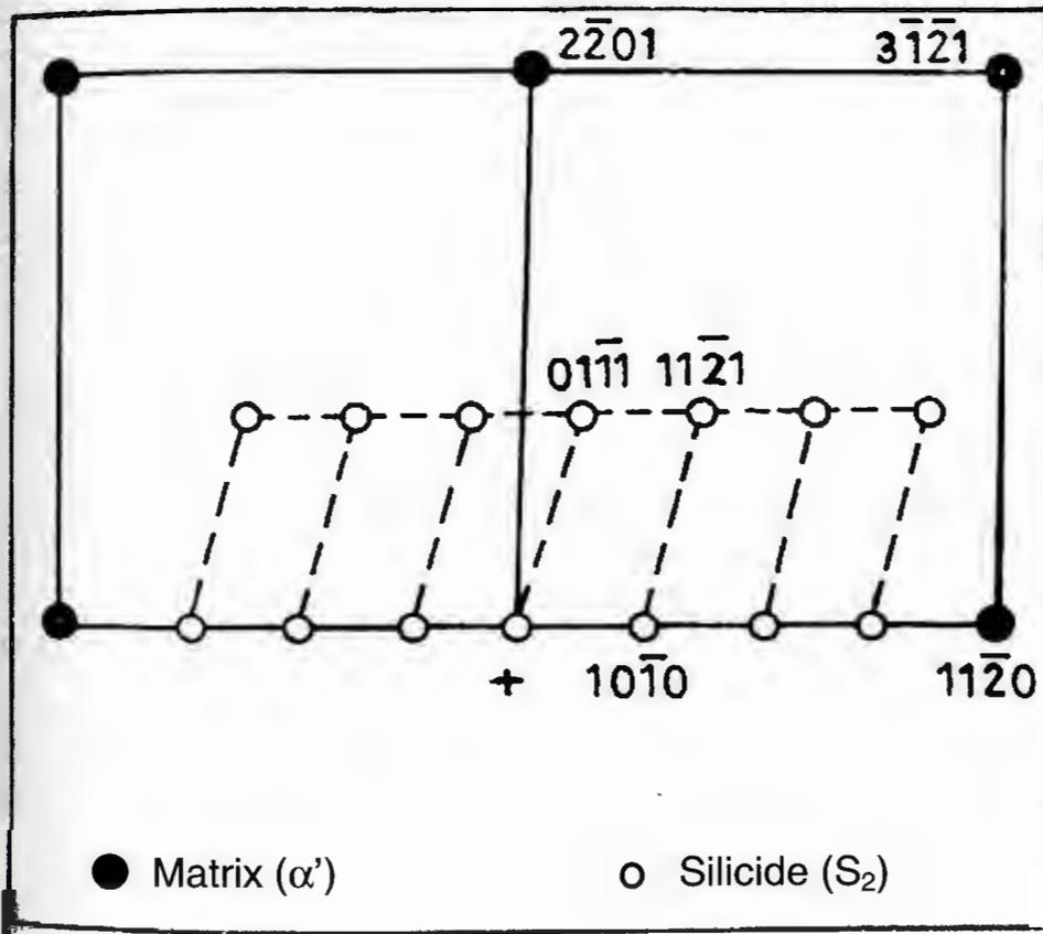
Figure 3-5: Schematic representation of TEM observations of IMI 829 aged for 24-hours at 700°C (from ref. [19]).
