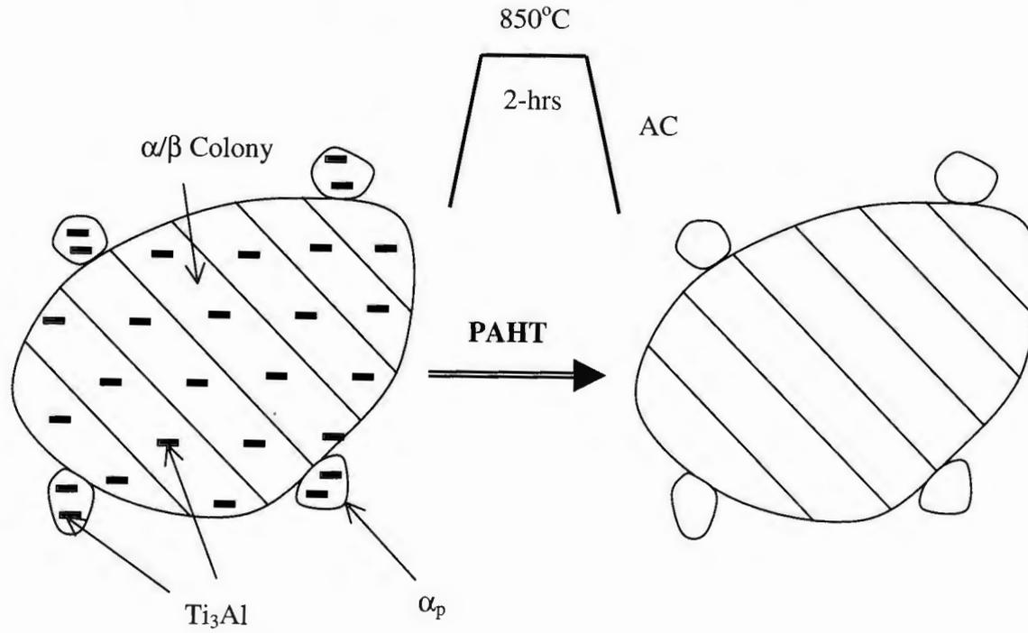
Figure 2-19: Schematic representation of Post Age Heat Treatment (PAHT) process in IMI 834.
