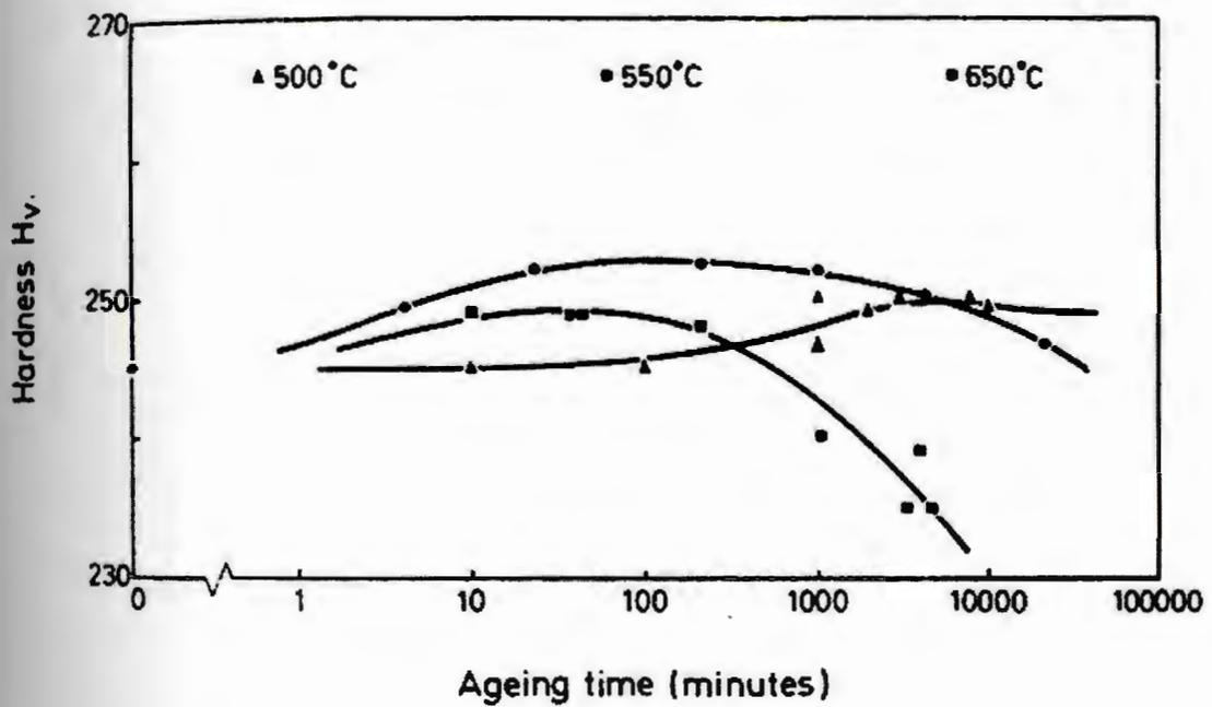
Figure 3-9: Effects of temperature on the aging characteristics of Ti-1%Si (from reference [45]).
