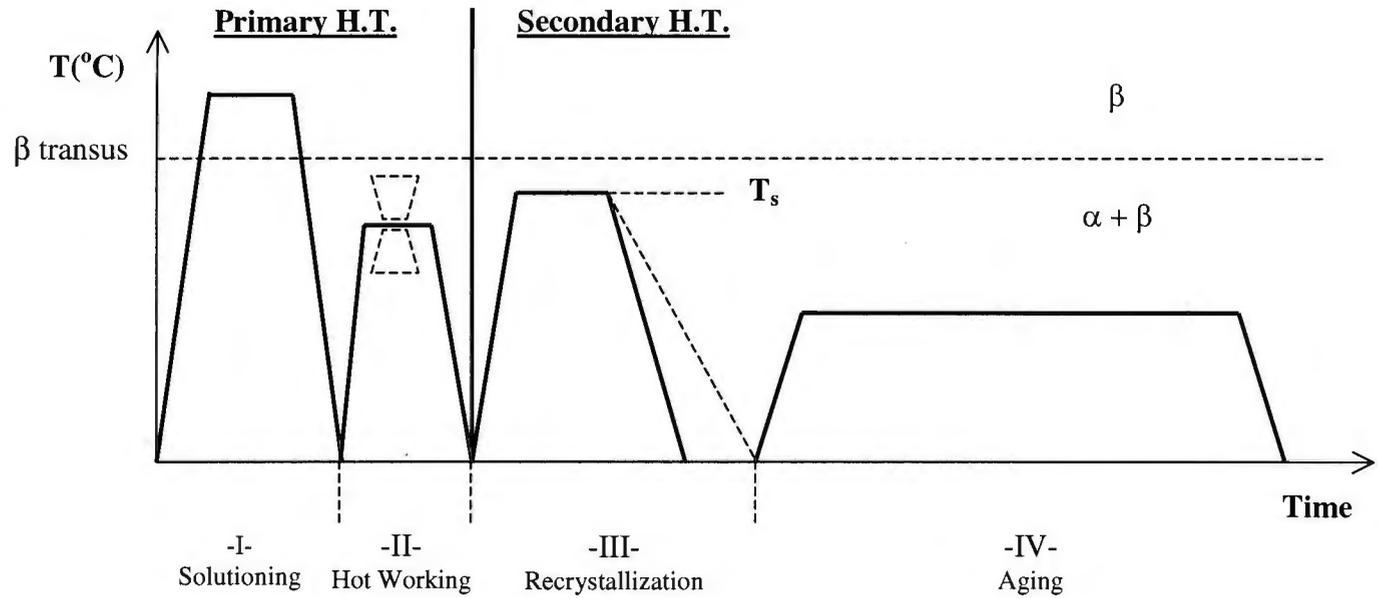
Figure 2-7: Thermal cycle applied in duplex microstructures ( $\beta$  transus in IMI 834 occurs at approximately  $1060^{\circ}\text{C}$  [21]).
