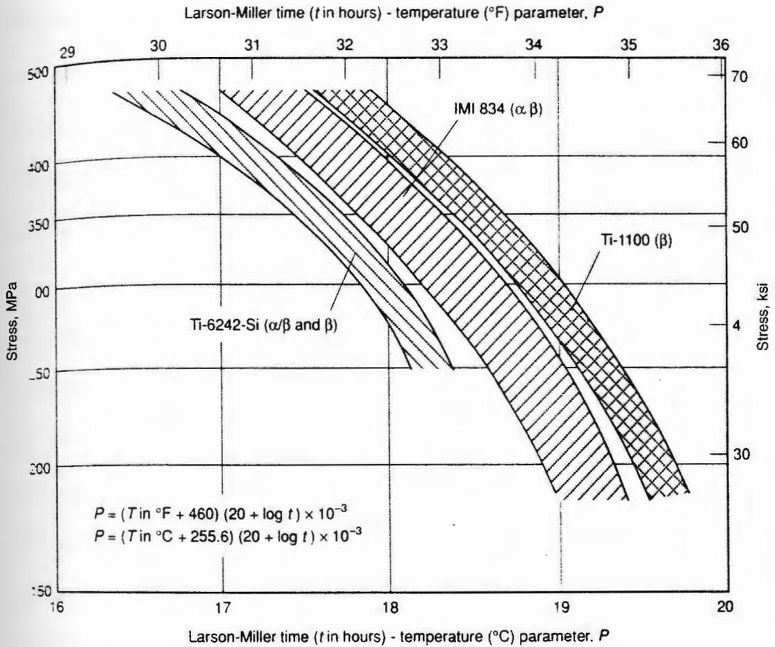
Figure.2-5: Creep properties in Ti6242 alloy, IMI-834 alloy and Ti-1100 alloy with  $\alpha/\beta$  and  $\beta$  processing as indicated (from ref. [8]).
