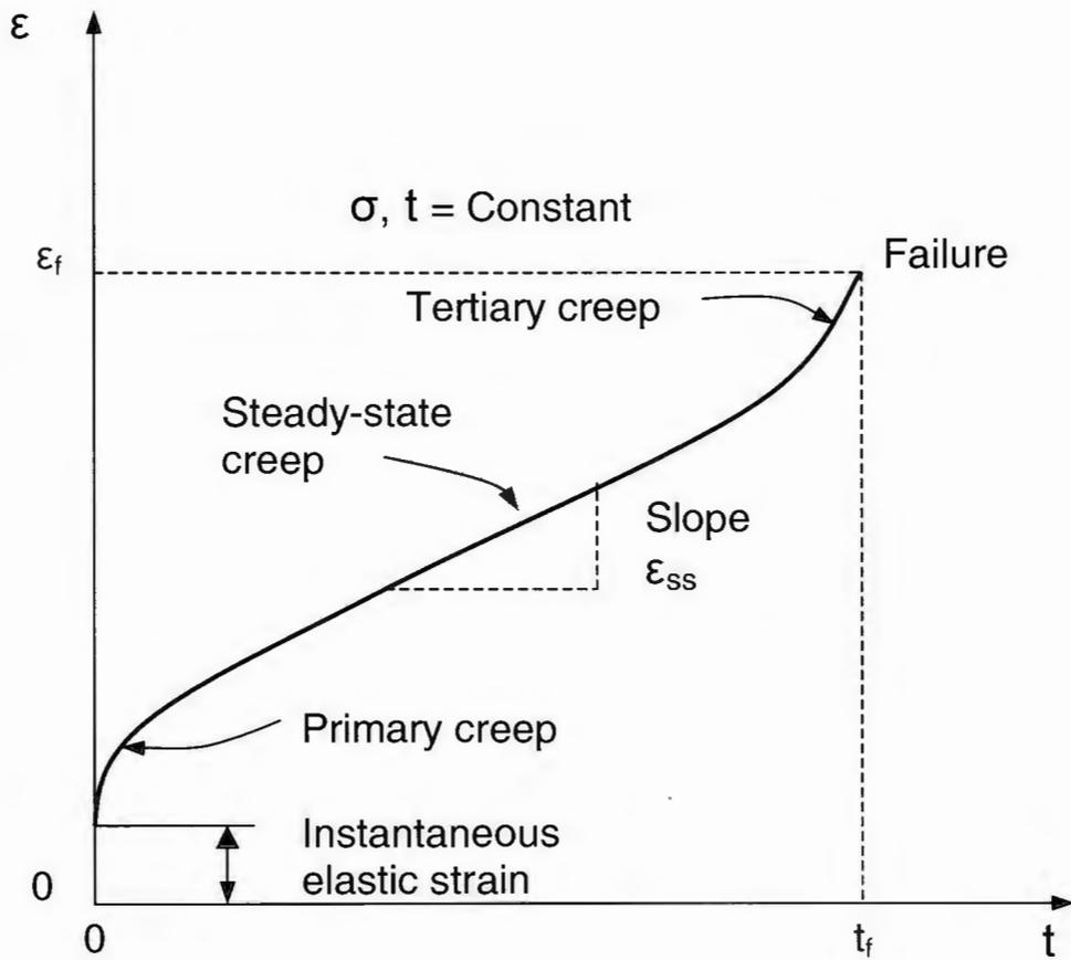
Figure A-1: Typical shape of a creep curve
