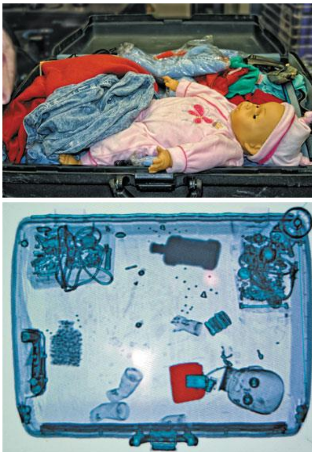
Figure 3: (top) photograph of what seems to be typical luggage. (bottom) CT image of the same luggage as above. The doll in the top image is an IED containing explosive that is highlighted in red by the CT image below [27].
