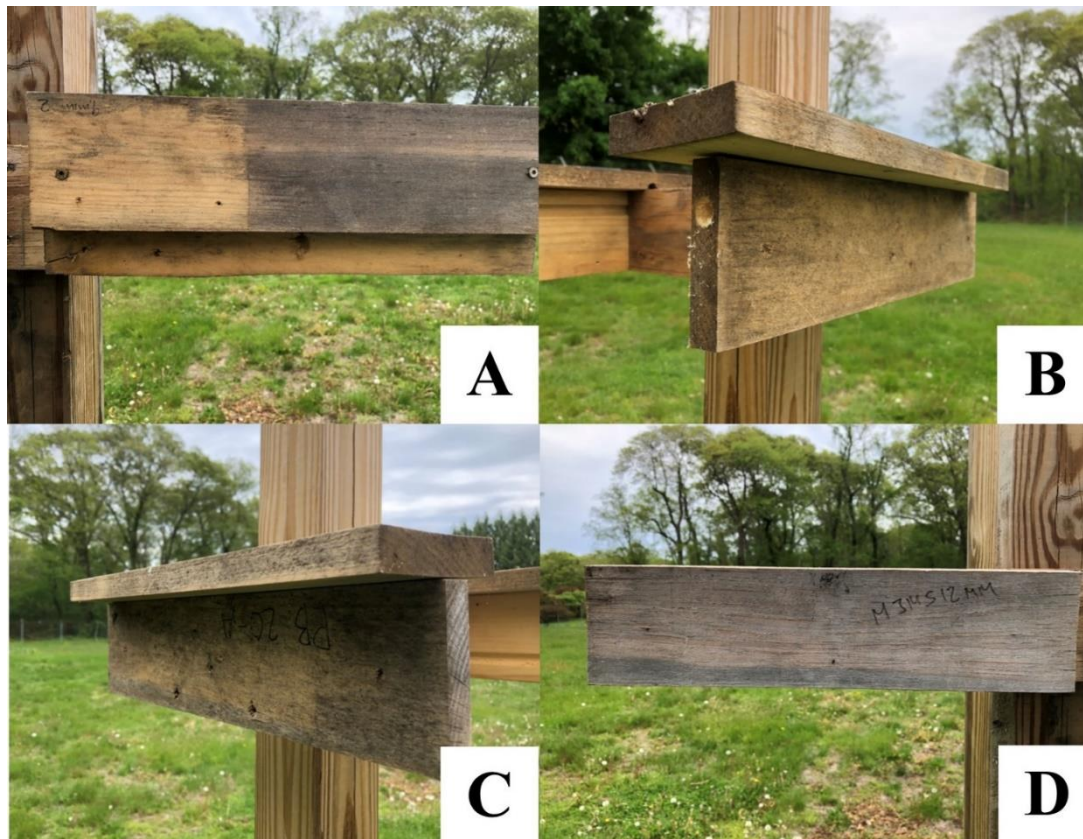
Figure 5. Manufactured nests attached to posts, 2018. A) Two pieces of weathered pine boards (36.5 x 2 x 9 cm) were overlapped in the middle and attached with screws. A 12 mm. diam. entrance hole was drilled in the middle of the boards just below the top board at a 60° angle and 2 cm deep. B) Two pieces of weathered pine boards as above were attached at right angles with a 15 mm overhang at the entrance end. The entrance was 12 mm in diam. and 3 cm deep. C) Two pieces of weathered pine boards as above were attached with screws at right angles. D) Weathered pine boards as above were routed in each of two boards to create two halves of 12 mm tunnel widths 15 cm long on each side of a 12 mm diam. entrance hole 15 mm deep.
