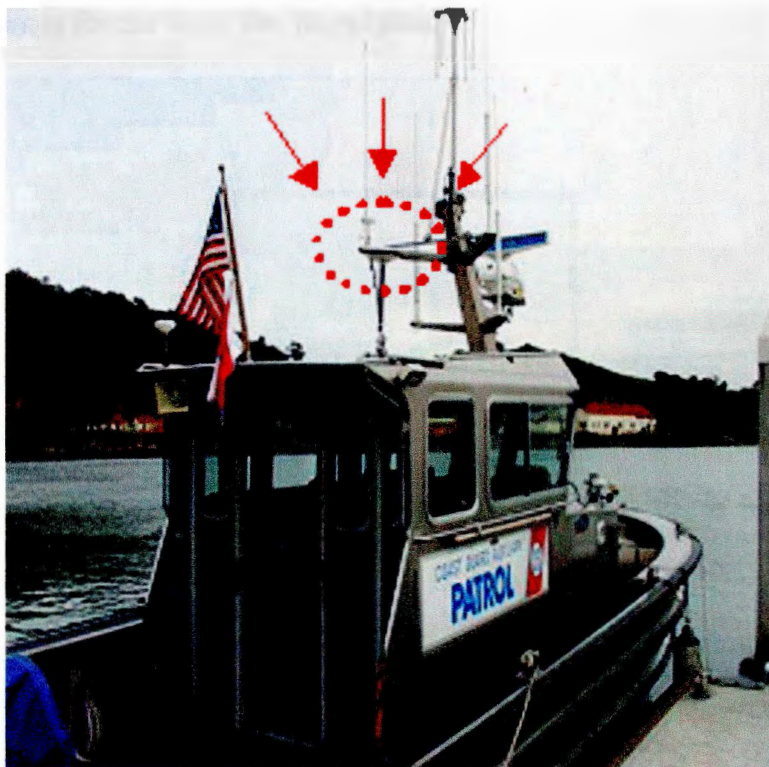
Figure 4.16 – Antenna location on research vessel.
