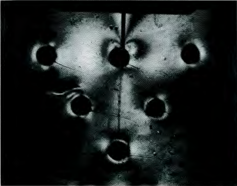
Figure 8. Photo 5/20 of isochromatic fringes as a dynamic crack intersects a Buna-N particle
