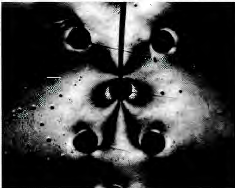
Figure 13. Photo 15/20 of isochromatic fringes as a dynamic crack intersects a Buna-N particle
