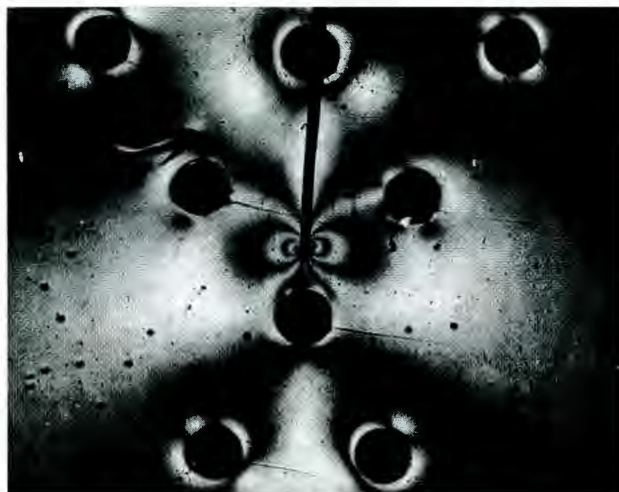
Figure 11. Photo 12/20 of isochromatic fringes as a dynamic crack intersects a Buna-N particle
