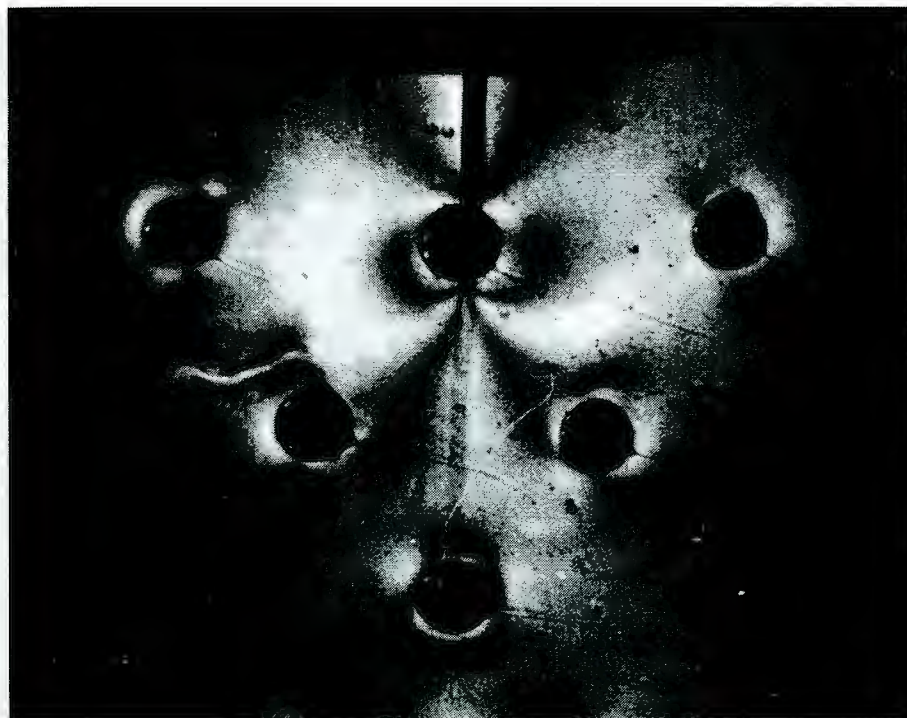
Figure 10. Photo 9/20 of isochromatic fringes as a dynamic crack intersects a Buna-N particle
