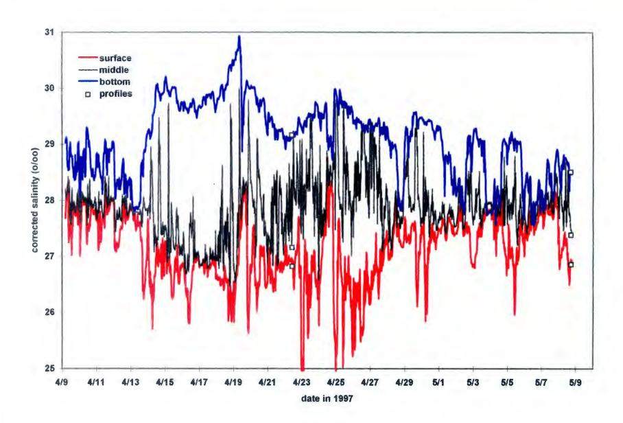
follows the features at the surface. Clearly the dominant feature, however, in the salinity record is the stratification on 13 April, in which deep salinity climbed by 2 0/00 and the surface dropped by about 2 0/00, in a few brief hours.
