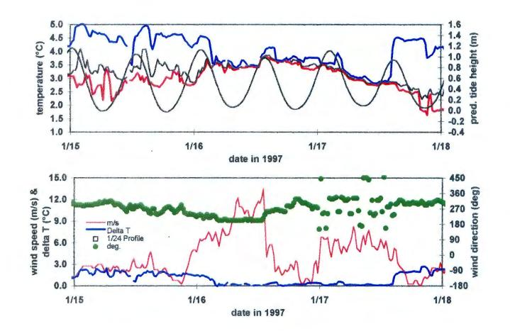
Temperature variations show pulses of warm water at the bottom instrument (Figure 43). These warm water pulses occur during high tides and are quickly mixed to lower temperatures during the outgoing tides. The rapidity of change of the bottom temperature increase during the flood is suggestive of an advective process rather than a mixing event. It is also interesting that the local low temperature at the bottom occurs at the end of the ebb, but prior to, slack low water.
