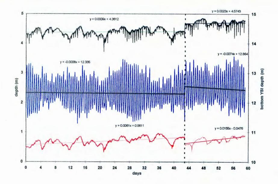
Figure 29. Corrected pressure data from three depths versus  $\Delta t$ , corrected using the drifts from Figure 40 and the calibration offsets. The surface and middle instruments' data are plotted on the left-hand y-axis, and the bottom instrument data is on the right-hand y-axis.
