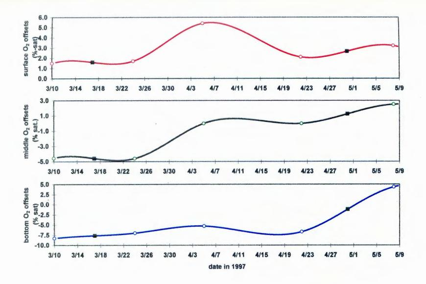
Figure 26a and b. Corrected dissolved oxygen at three depths, 0.5-m, 4.4-m, and  $\sim$ 12.6-m, as measured, in twenty minute intervals, by the three YSI-600XL's attached to the buoy.
