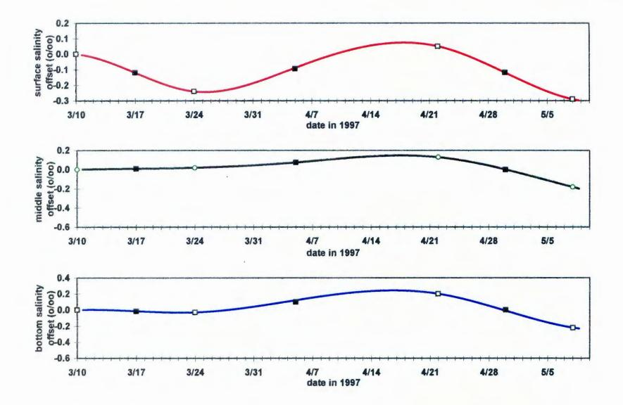
Figure 22a and b. Corrected salinity at three depths, 0.5-m, 4.4-m, and ~12.6-m, as measured, in twenty minute intervals, by the three YSI-600XL's attached to the buoy.
