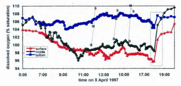
Figure 24. Dissolved oxygen as recorded by the surface, middle and bottom instruments. The data marked as "+" markers are raw data, and the filled squares indicate the corrected data, having been incrementally offset to remedy the drift as indicated in Figure 23. The profiles 2, 5, and 7, at noon, 14:15 and 15:30, respectively, are marked with the readings at the depths of the buoy instruments marked as "S", "M" and "B", for surface, middle and bottom.
