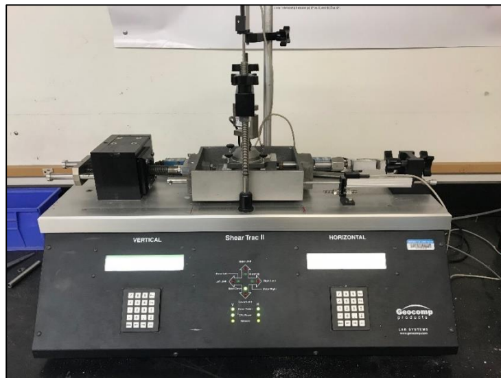
Figure 10: Photograph of the Geocomp direct shear test device.
