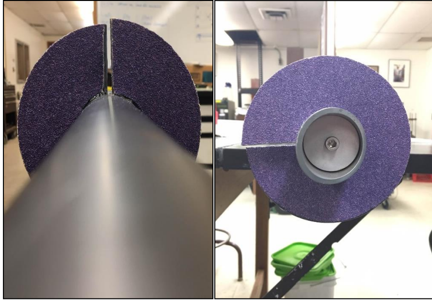
Figure 16 – Photograph of the anchor with sand paper attached to the helix plates.
