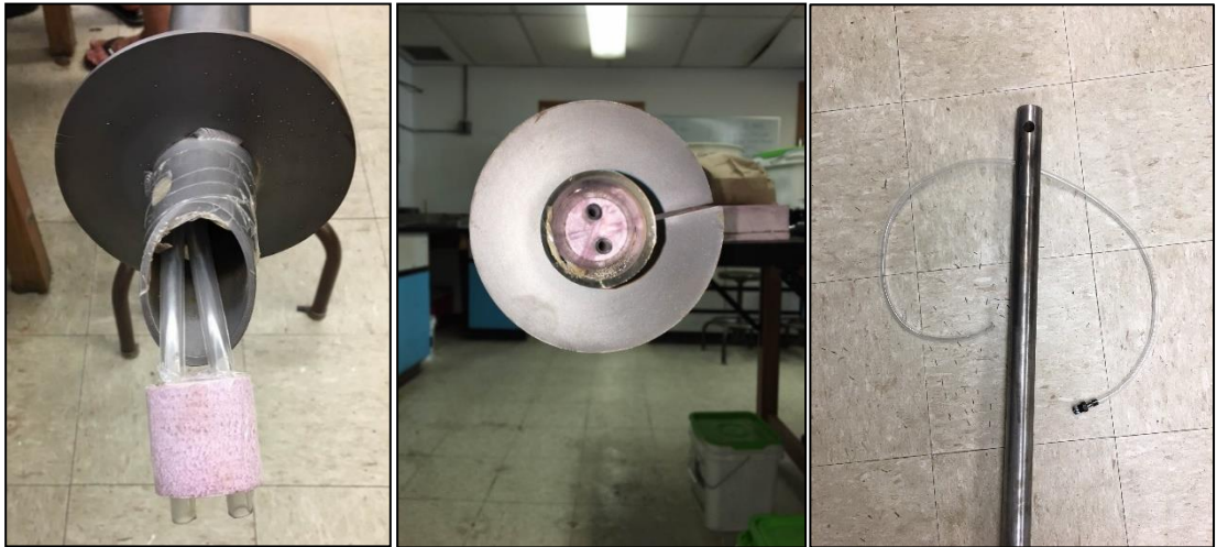
Figure 18 – Photograph of the anchor with vacuuming / jetting equipment attached.
