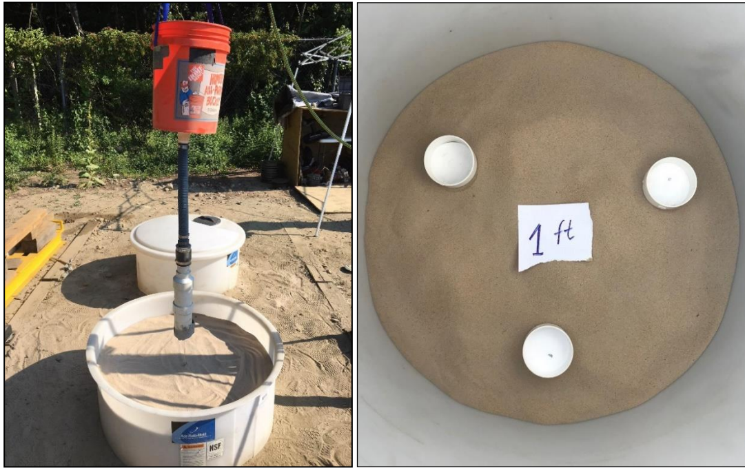
Figure 12 – Photographs of (a) pluviator device and sand tank (b) sand containers before pluviation
