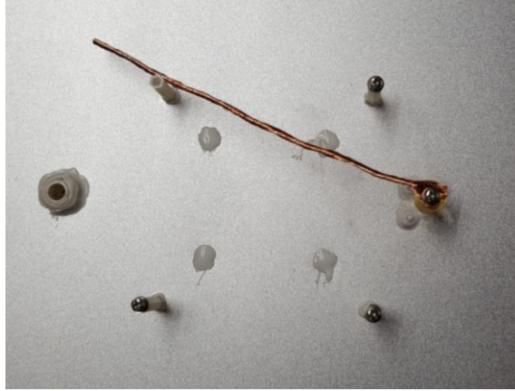
Figure 13 Copper Monopole Antenna
