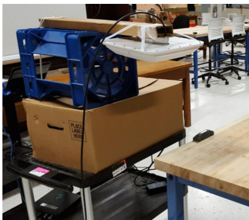
Figure 22 Construction of the movable Antenna
