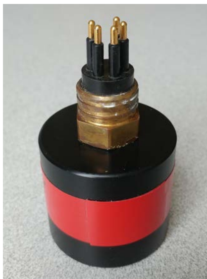
Figure 28 Final single-cylinder hydrophone
