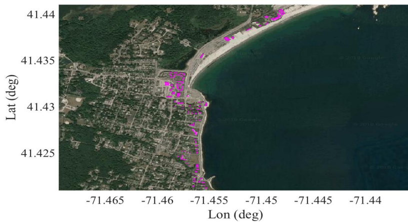
Fig. 1.10. FUNWAVE Obstacle locations have been highlighted on Google Earth (Google, 2018). Obstacle points identify spots on the grid that remain dry (building with foundations).
