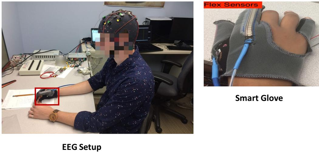
Figure 12. The Subject with EEG electrodes placed in his head is shown in the figure. The subject is also wearing the Smart Glove in his right hand. The Smart Glove is also shown in the figure .
