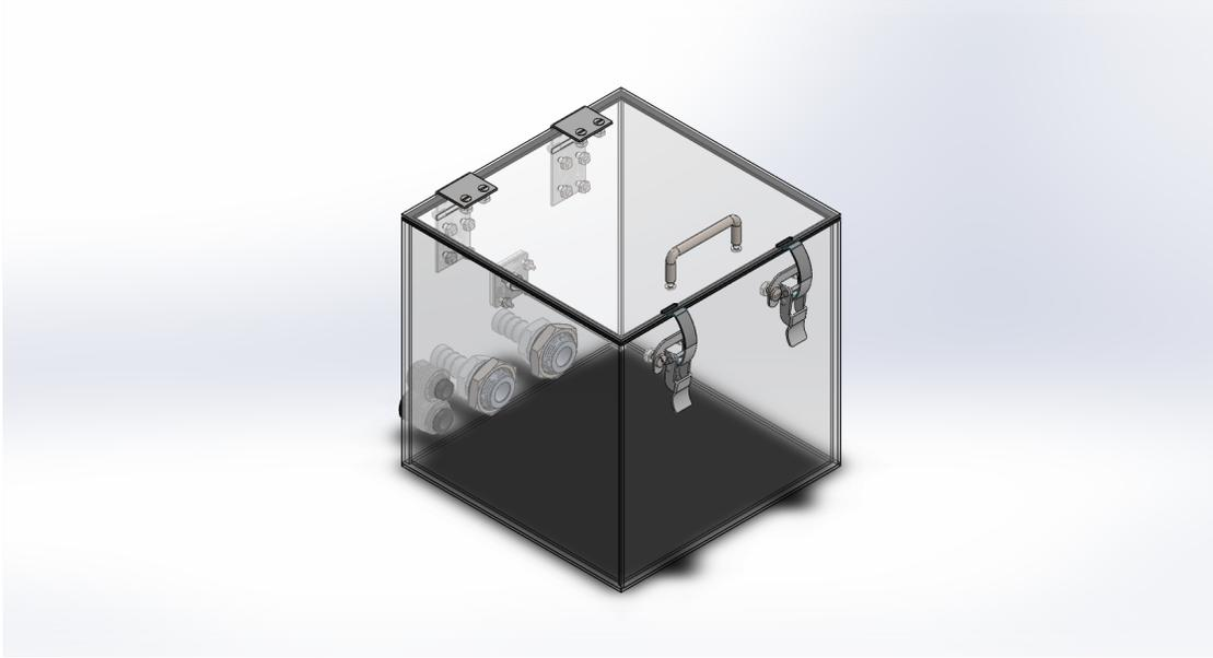
Figure 3.2. 3-D CAD model of enclosure assembly without heaters or humidifier.
