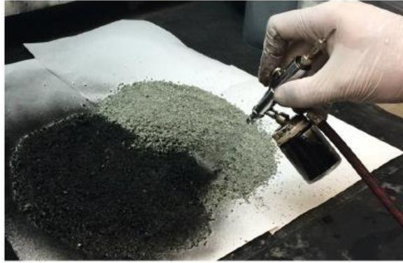
Figure 16 Spray painting of conductive MWCNT-latex ink onto fine aggregates
