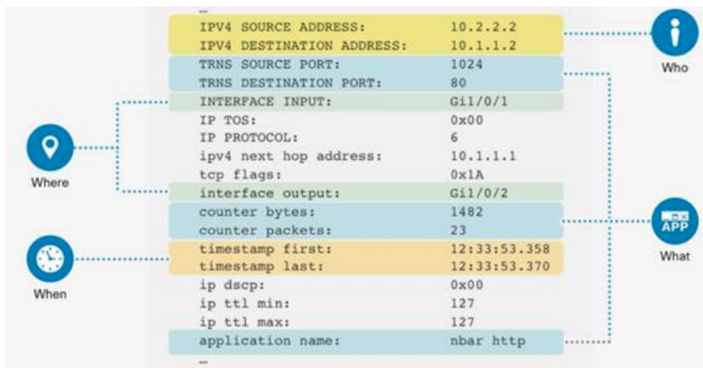
Figure 3A – NetFlow Attributes (Log Fields) - NetFlow Record Provides a Significant Amount of Information (Courtesy of CISCO)
