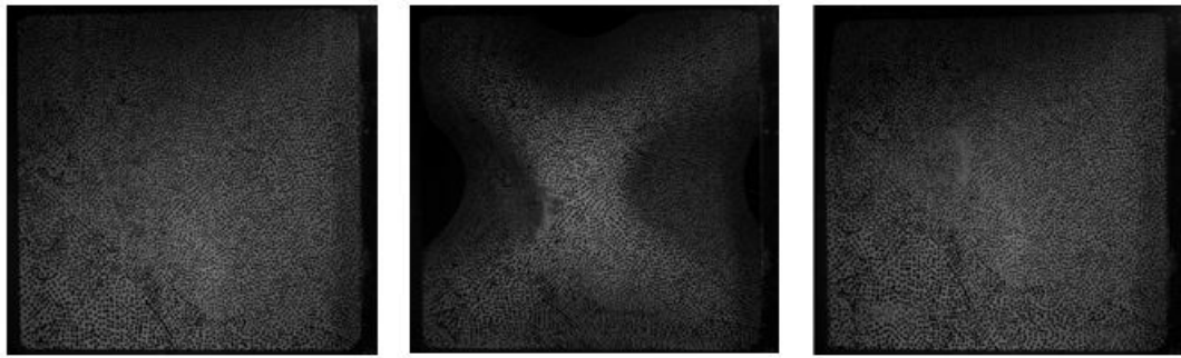
Figure 44. 60-9c panel images before, during, and after blast using high speed cameras
