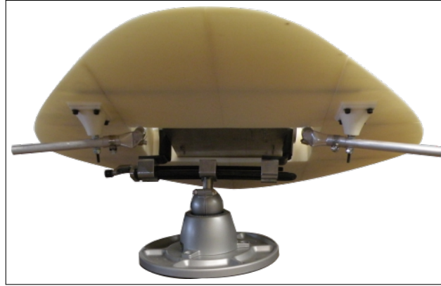
Figure 3.1.8: Image of bottom of vehicle prior to sealing and painting, showing the underwing mount points for the legs
