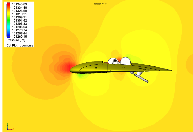
Figure 4.6.4: Pressure field when the vehicle is in a uniform flow with zero angle of attack
