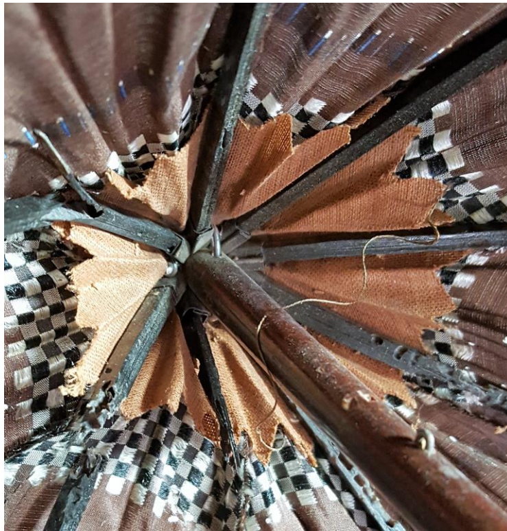
Figure 13: The inside of the parasol where the ribs meet at the stick. This image shows whalebone ribs with severe insect damage that have ends wrapped in thin metal that have been drilled through with a wire binding them all together and also looping through the stick itself. Photograph by author. (Accession #: 1950.01.111)
