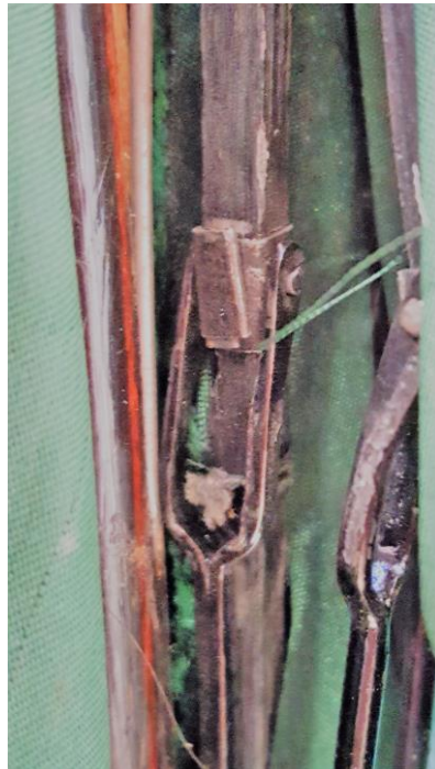
Figure 14: A square whalebone rib is wrapped in metal with the forked metal stretcher meeting it, and a pin through the metal and rib holding the two together. Photograph by author.
