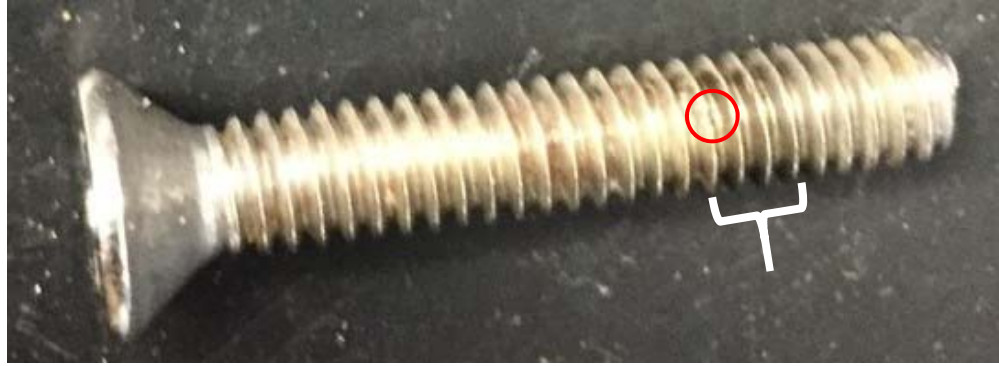
Figure 17: The stainless screw from sample SS2 after it was extracted from the CFRP panel and any remaining sealant was carefully removed. Note the slight blackened area, indicated by the bracket. The blackened area is where the screw was in direct contact with the CFRP. Additionally, there appears to be a roughened area on one of the threads, as indicated by the red circle. This roughened area may be a sign of corrosion damage. Picture is courtesy of Jordan A. Ortiz.
