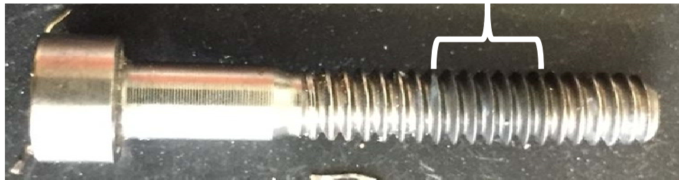
Figure 9: The titanium screw from sample Ti2 after it was extracted from the CFRP panel and had any remaining sealant carefully removed. Note the apparent lack of any corrosion-related damage as well as the presence of a slight blackened area, indicated by the bracket. The blackened area is where the screw was in direct contact with the CFRP. Picture is courtesy of Jordan A. Ortiz.
