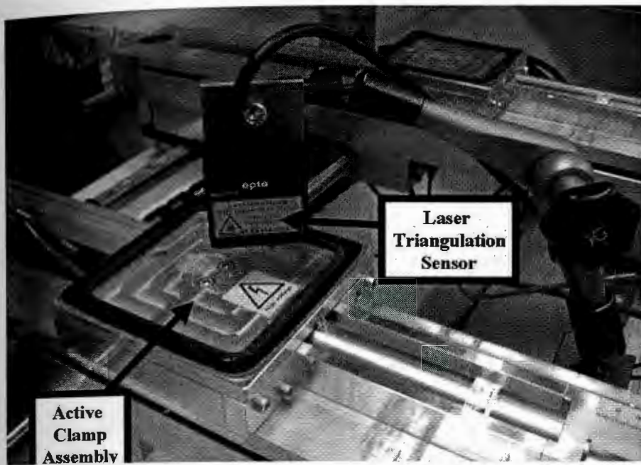
Figure 2.6. Test Setup with Laser Triangulation Positioning Sensor
