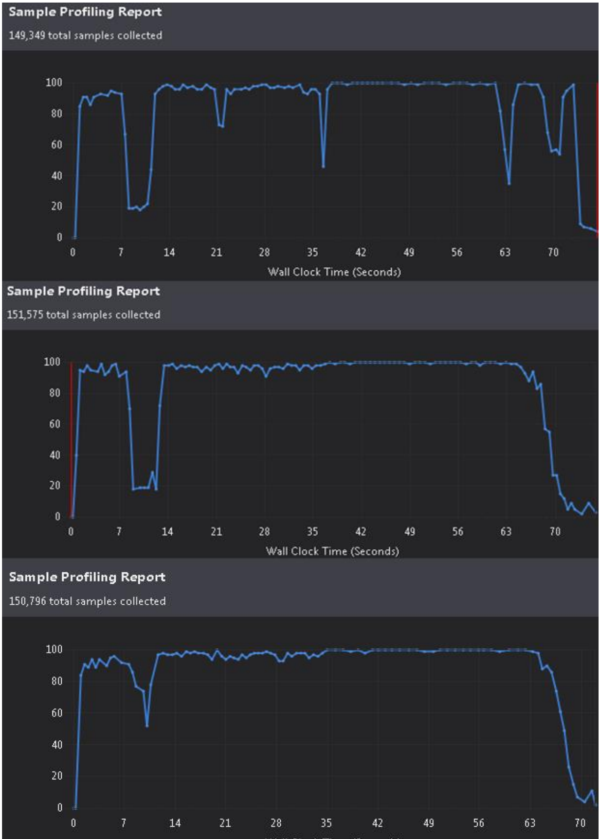
Figure 8: From top to bottom shows a 92, 95 and 97 percent parallel program's CPU utilization
