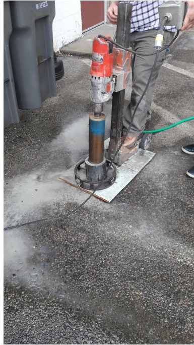
Figure E-3 Sample being cored to required test diameter.
