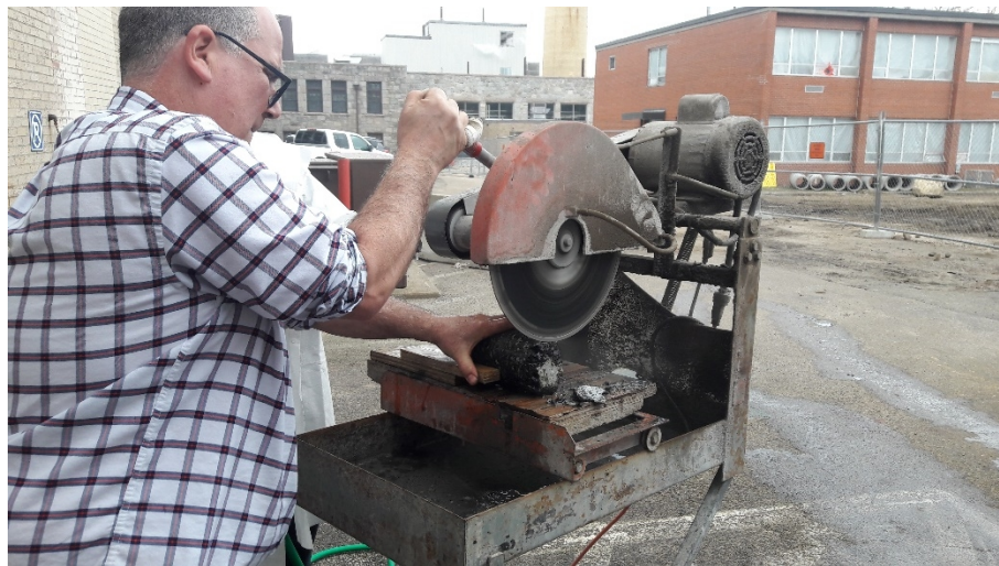
Figure E-4 Sample being sawed to obtain parallel faces.
