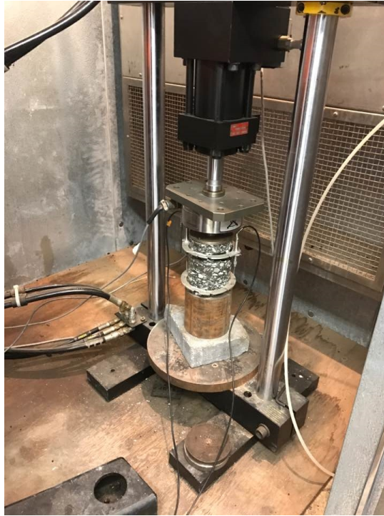
Figure E-8: Specimen along with a Jig to fix LVDTs
