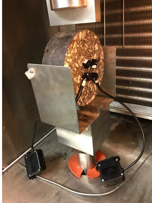
Figure D-3: Specimen inside the Loading Frame Chamber of Instron Machine
