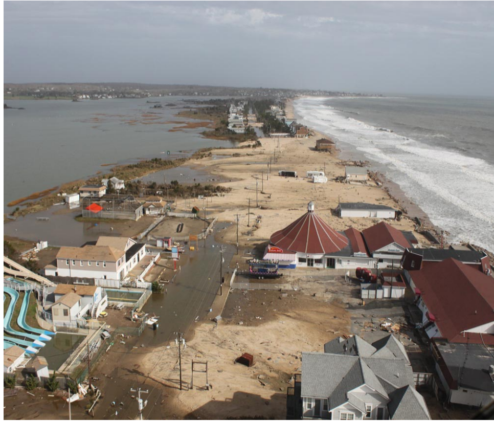
Figure 5: Overwash in Misquamicuit, Rhode Island after hurricane Sandy. Photo: Rhode Island Department of Transportation
