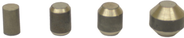
Figure 3: \text{Ti}_2\text{AlC} specimens, from left to right: unconfined, low confinement, medium confinement, and high confinement.
