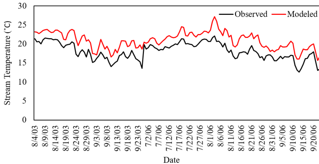
Figure 6: A hydrograph of the Queen River stream temperature modeled versus observed 2003 and 2006. The modeled stream temperature is produced using the hydroclimatological model and the observed data was collected by the Wood-Pawcatuck Watershed Association. With minimal observed data it was not possible to produce satisfactory calibration results.
