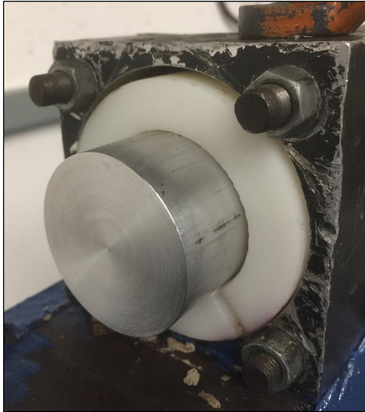
Figure 34 – Aluminum striker centered within gas gun by O-rings
