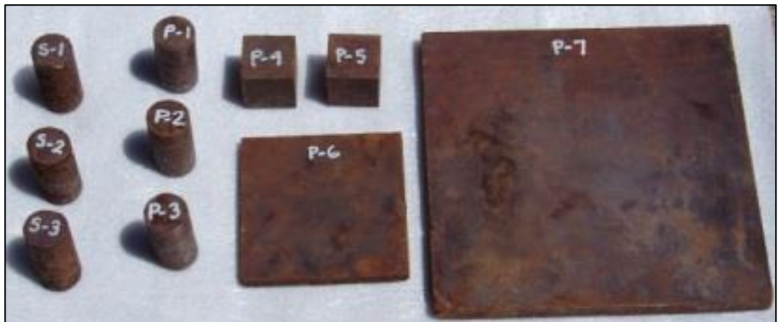
Figure 29 - Samples provided by Iron Shells LLC. P-series contains polypropylene fibers; S-series contains steel fibers
