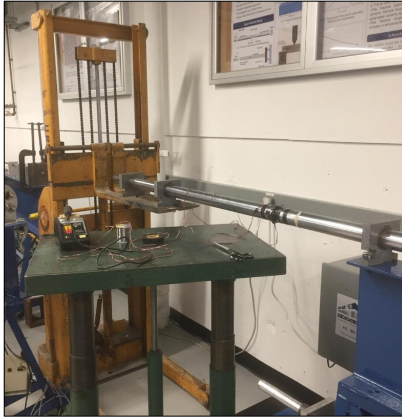
Figure 35 - KWIK-STAK portable elevating truck to support the overhanging part of the SHPB system
