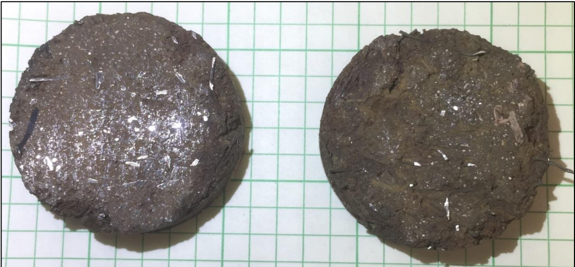
Figure 31 - Steel fiber containing samples („S1“-series) cut with a diamond saw blade (left) and with a steel saw blade (right)
