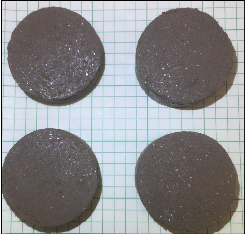
Figure 30 - Cut and smoothed samples from „P1“-cylinder
