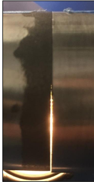
Figure 40 - Gap between incident bar (left) and transmitted bar (right) indicating misalignment
