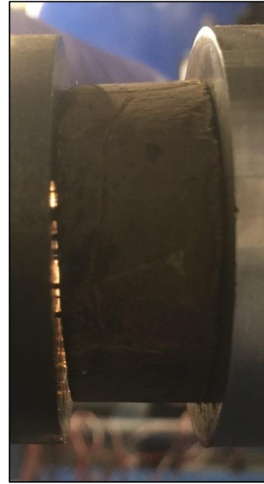
Figure 64 - Misalignment of Iron Carbonate specimen P1-2
