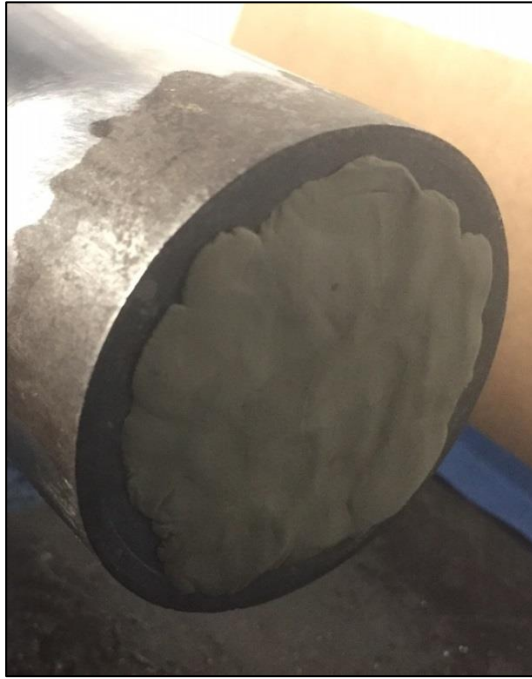
Figure 63 - Clay as pulse shaper on one face of the incident bar
