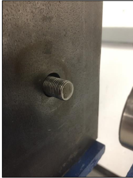
Figure 18 - Clay as pulse shaper on an 0.5 in. incident bar at the Dynamic Photomechanics Laboratory
