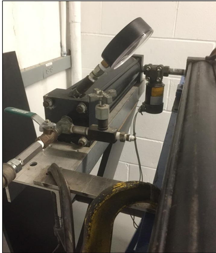
Figure 42 – Repositioned pressure regulator with short connector mounted on the SHPB stand
