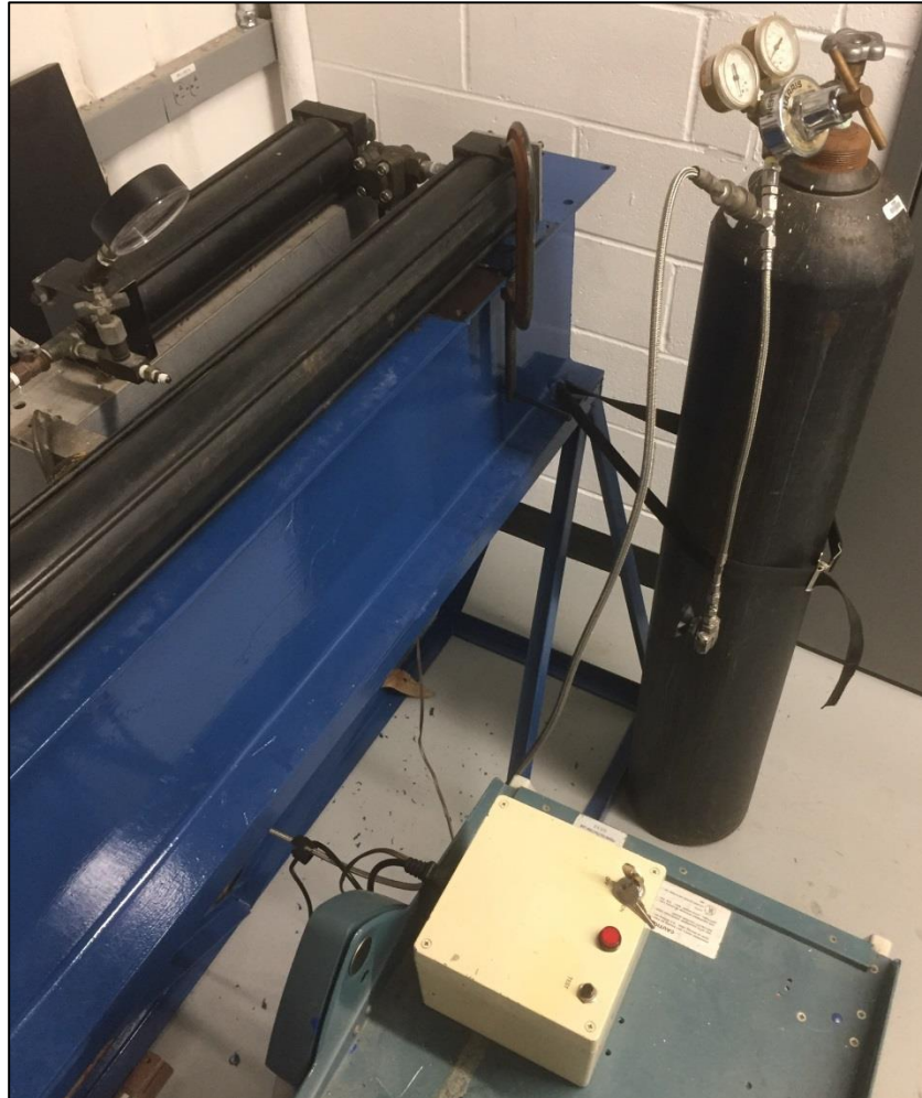
Figure 36 - compressed gas mechanism with gas tank, automatic gas launcher, and solenoid valve control box
