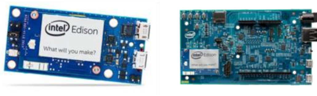
Figure 4. Intel Edison Fog Computing Board (Left: Edison with the Mini breakout kit, Right: Arduino Breakout kit with the Edison)
