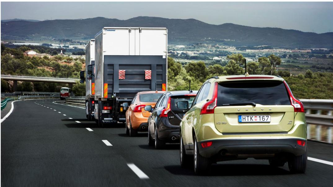
Figure 8: A mixed vehicle platoon in the SARTRE project
