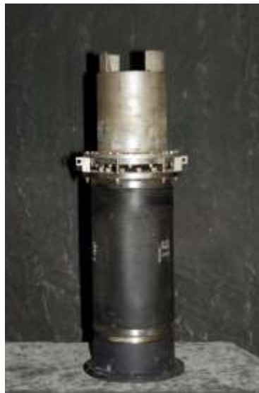
Figure 8: The HX-29 bender bar projector. (Image source: USRD acoustic augmentation support program (AASP))
