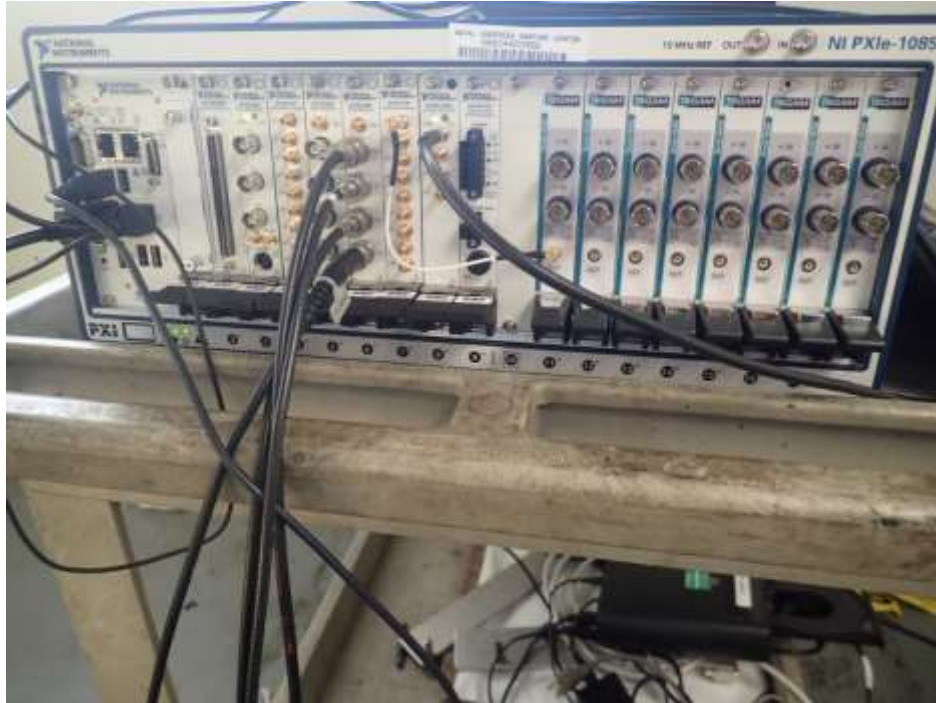
Figure 29: A picture of the PXI chassis that records the experimental data. Four channels with recorded on the PI-4462 card: acceleration, command voltage, voltage across the MMA's coils, and current applied to the actuator.
