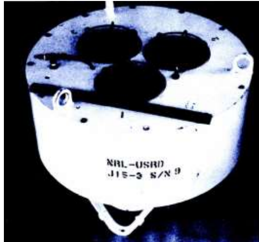
Figure 6: The USRD J15-3 moving coil projector. (Image source: [8])
