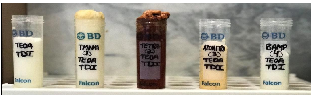
Figure 2.19 Expansion of foams, from left to right: TEOA-TDI, TMNM(1)/TEOA-TDI, TETRA(2)/TEOA-TDI, AZONITRO(3)/TEOA-TDI, BAMP(4)/TEOA-TDI
