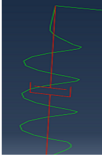
Figure 7. Zoomed in view of the Abaqus Spring-Dashpot Model
