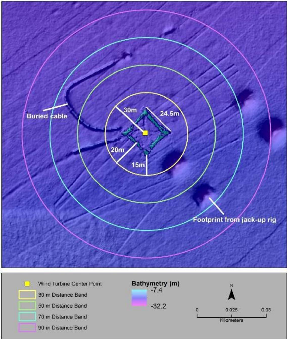
Figure 18. The relationship between the distance bands and footprint of the foundation structure. Turbine 5 is shown here and is also representative of Turbines 1 and 3. *Note: Multibeam data provided by Fugro USA Marine, Inc (Fugro, 2017).*
