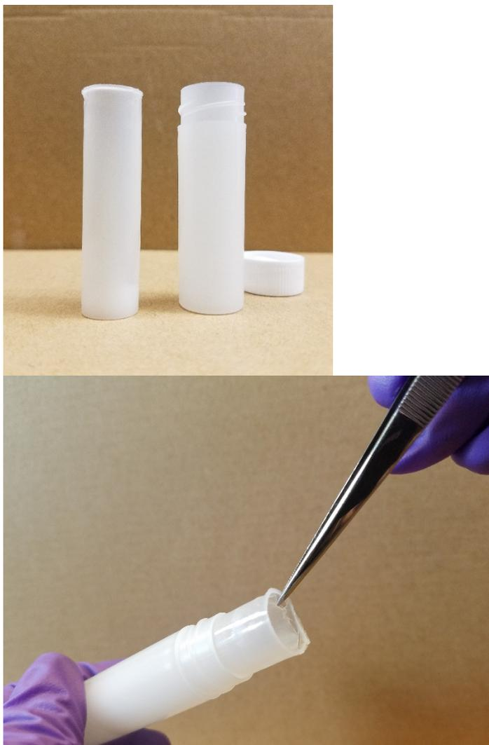
Figure 4.6. Solvent-free ROP allows for the direct-from-monomer creation of a negative mold in seconds. Above, the hollow, PVL negative mold is of a polypropylene reaction vial. Conditions: 10 mmol VL, 0.049 mmol TCC/BEMP (each), 0.020 mmol benzyl alcohol (see Experimental Section).
