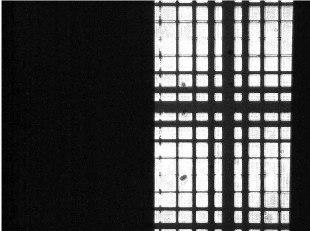
**Figure 2. Optical system polarization.** When the external polarizer rotates to the vertical orientation, the vertically signal will completely pass the filter (right side), while the horizontally signal completely being blocked by the filter (left side).
