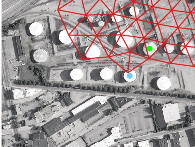
Figure 15. Example of a point with three adjacent nodes (green) and point beyond the nearest wet node (blue). The red lines represent wet portions of the unstructured ADCIRC grid. Points tested are both inside and outside of the grid, and constrained by a basin analysis.
